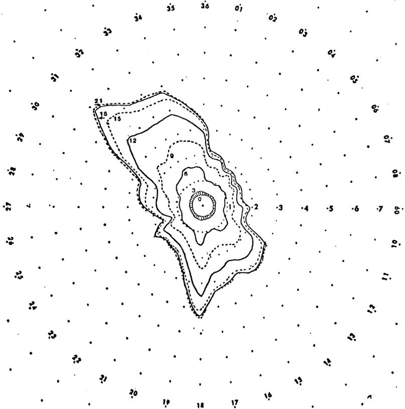
NOTE: wind speeds are shown in knots on all isopleths. Divide by 2 to obtain meters/sec.
