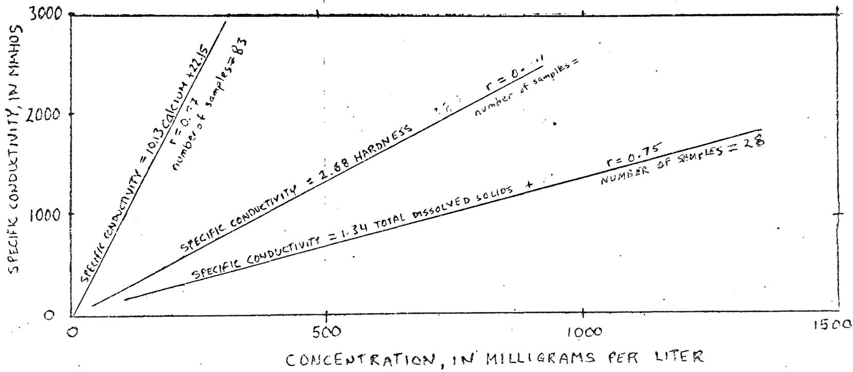
FIGURE . . . Graph showing relation between specific conductivity and selected constituents in ground water collected from the Copper-Nickel Study Area.
