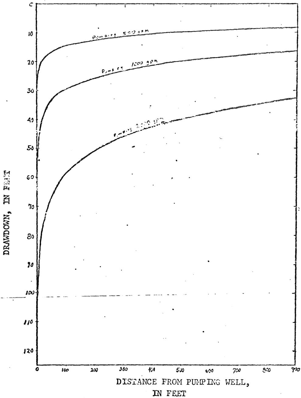
Figure Distance-drawdown curves for a well pumping from the aquifer underlying the Embarrass River
