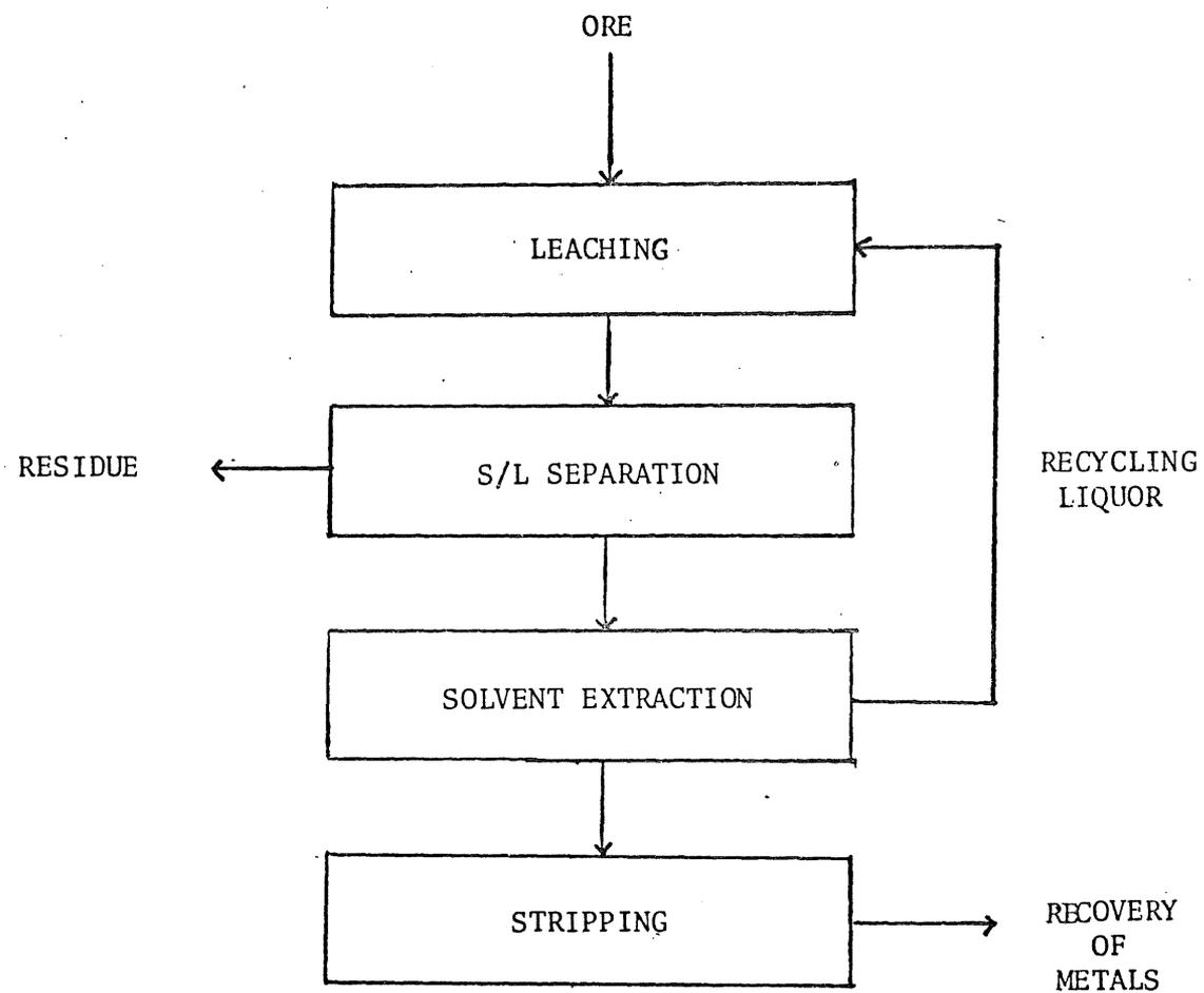
Fig. 22. Simplified flowdiagram for bacterial leaching of ores and minerals.
