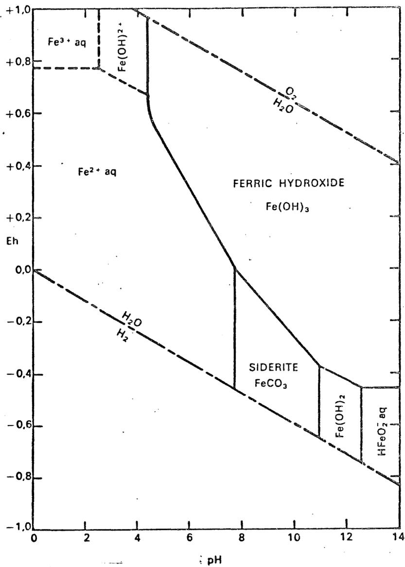
Fig. 11. Eh-pH diagram showing the relationship among metastable iron hydroxide species and siderite at 25°C and 1 atm total pressure. Concentration of dissolved species  $10^{-6}$  M. 50
