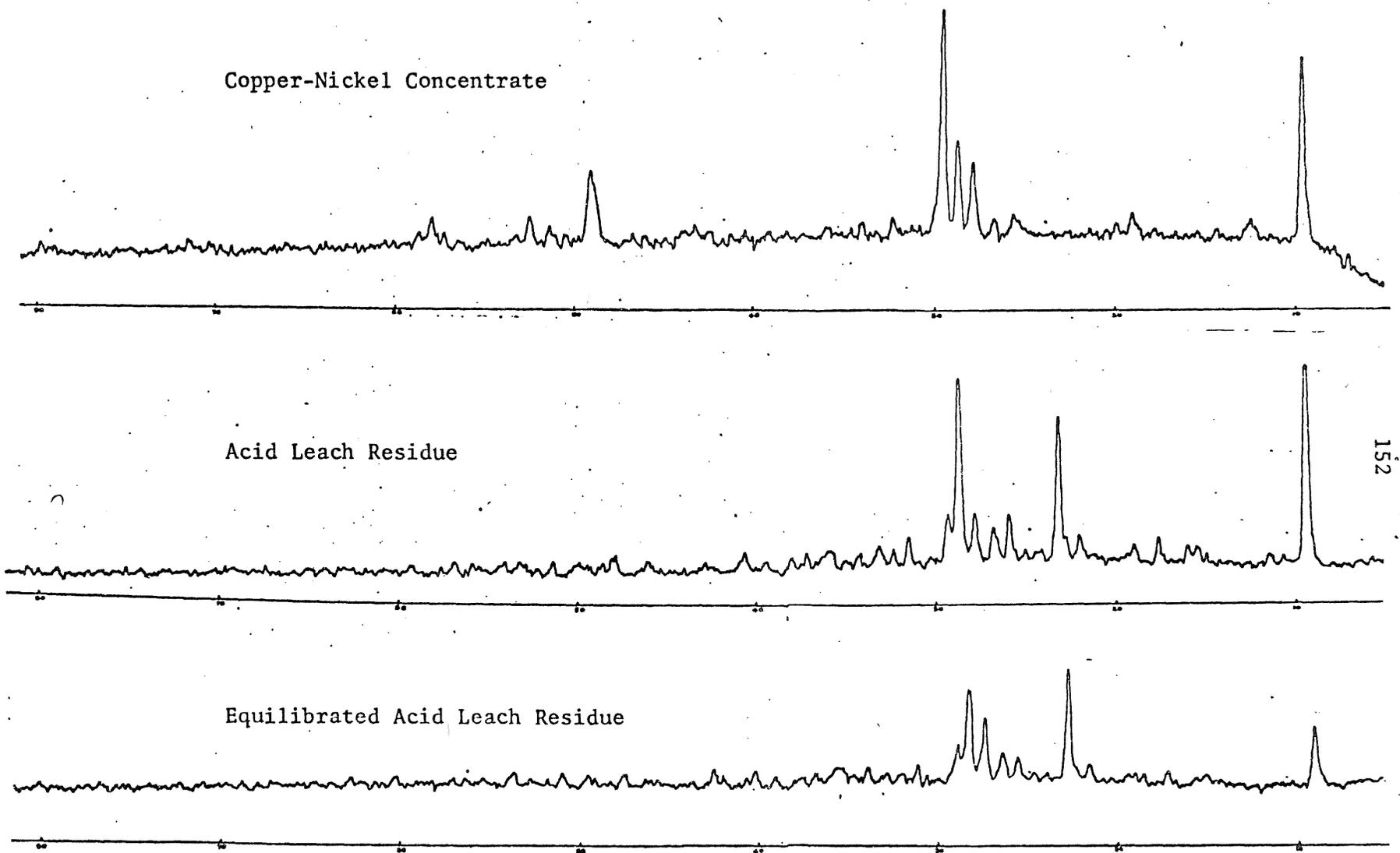
FIG. 52. X-RAY DIFFRACTOGRAPHS OF ACID LEACH RESIDUE, BEFORE AND AFTER EQUILIBRATION, AND THE CONCENTRATE
