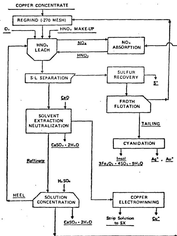
Fig. 17. Flowsheet for processing copper concentrates with nitric acid.<sup>73</sup>
