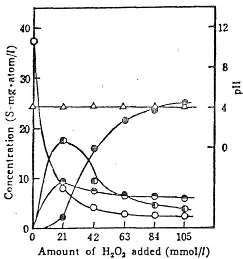
Fig. 47 Oxidation of sodium thiosulfate with hydrogen peroxide in the presence of iron 129
