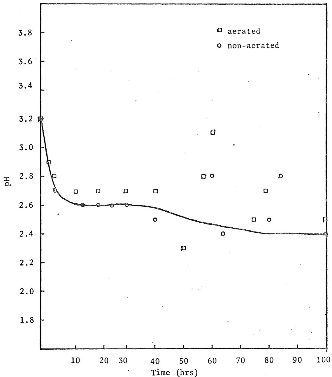
Fig. 55. Effect of aeration on equilibration of basic ferric sulfate
