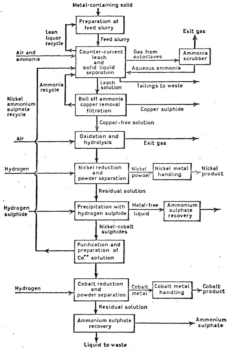
Fig. 1. Flowsheet for Sherritt Gordon process for production of nickel and cobalt metals from sulfide ore. <sup>158</sup>
