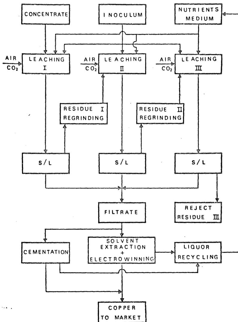
Fig. 21 Schematical representation of a microbiological batch leaching process for chalcopyrite concentrate treatment. 99
