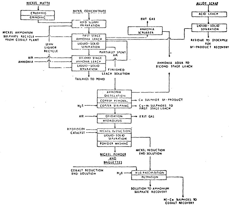
FIG. 5 SHERRITT GORDON MINES, LTD, SIMPLIFIED NICKEL REFINERY
