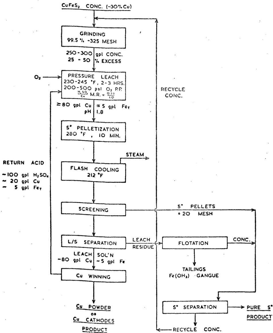
even at low levels of sulfuric acid additions, while copper required significantly higher levels of sulfuric acid additions to attain high extractions.
