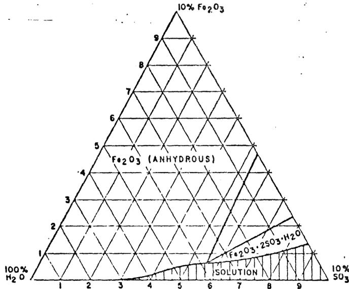
Fig. 26 System  $\text{Fe}_2\text{O}_3\text{-SO}_3\text{-H}_2\text{O}$ . Equilibrium at  $200^\circ\text{C}$  104
