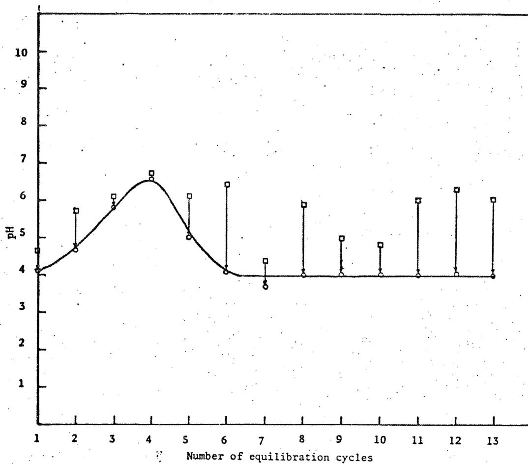
Fig. 50. Equilibration curve for acid leach residue
