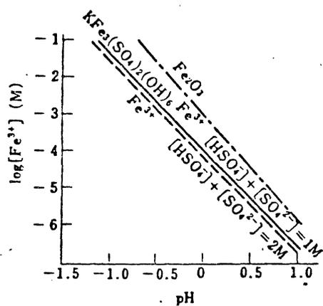
Fig. 37. Log[Fe<sup>3+</sup>] - pH relation in iron hydrolysis.<sup>113</sup>
