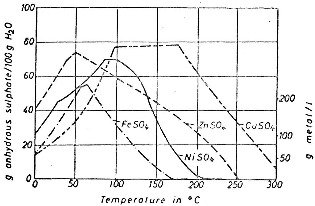
Fig. 41. Solubility of some metal- sulfates as a function of temperature.
