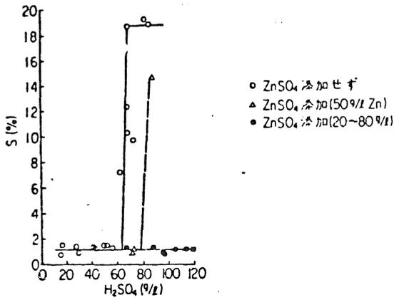
Fig. 27. Sulfur content in hydrolysis product as a function of free  $H_2SO_4$  (200°C) 117
