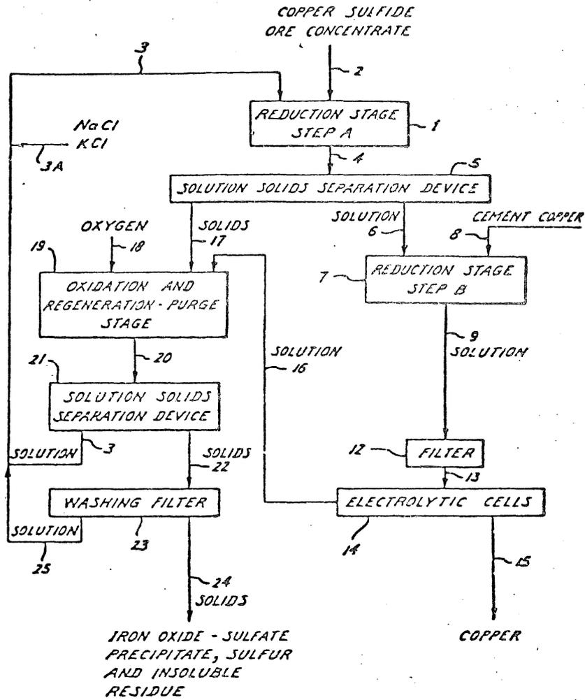
Fig. 14. DUVAL'S "CLEAR" PROCESS, 61
