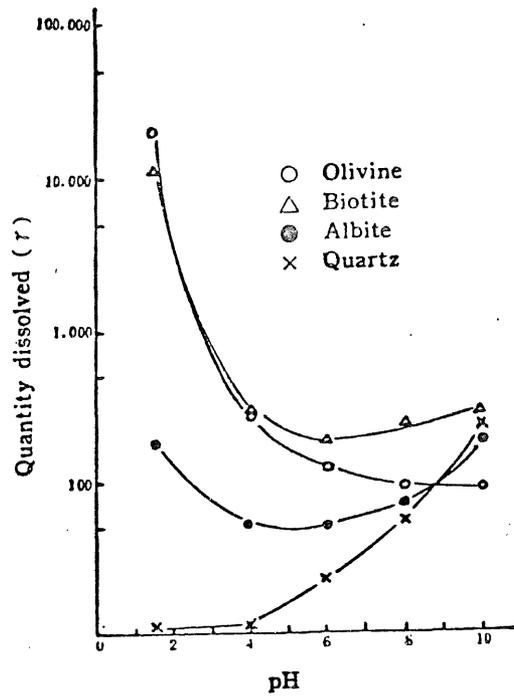
Fig 48. The relation between the minerals and the quantity of silica dissolved. 149
