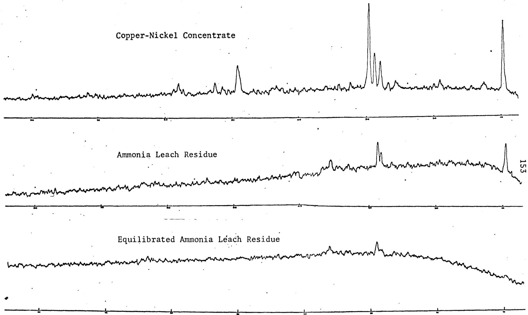
FIG. 53. X-RAY DIFFRACTOGRAPHS OF AMMONIA LEACH RESIDUE, BEFORE AND AFTER EQUILIBRATION, AND THE CONCENTRATE
