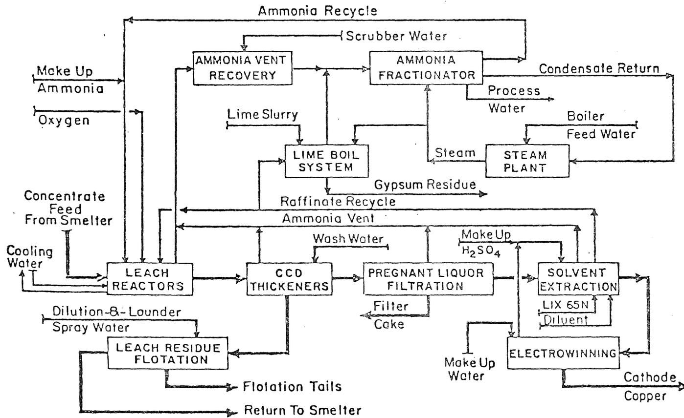
FIGURE 3.— Anaconda Arbitrator Plant — block flow diagram. 12
