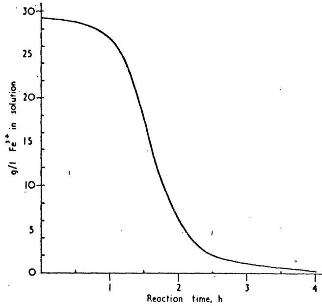
Fig. 40 Progress of precipitation of iron as jarosite. Solution: 29.1 g/l  $Fe^{3+}$ , 45 g/l  $H_2SO_4$  112
