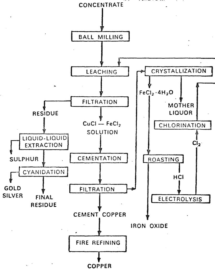
Fig. 12. Schematic flowsheet proposed by Haver and Wong for the treatment of chalcopyrite concentrates.<sup>60</sup>
