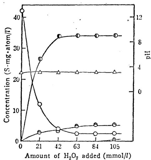
Fig.-46. Oxidation of sodium thiosulfate with hydrogen peroxide in an acidic solution 129
