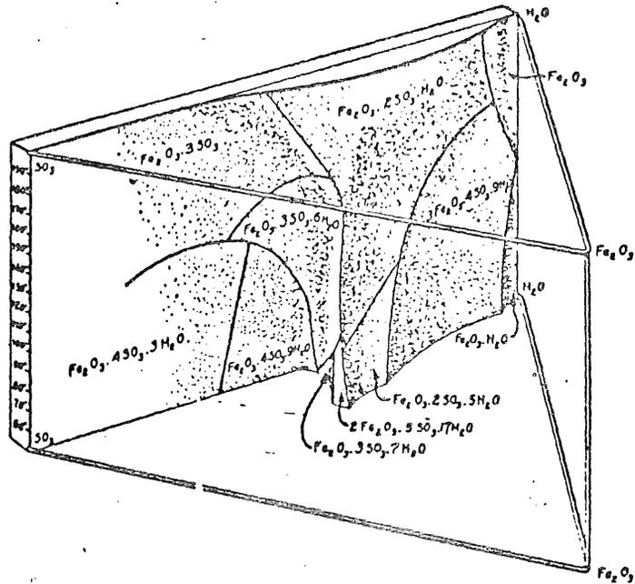
Fig. 23. Solid model of the system,  $\text{Fe}_2\text{O}_3\text{-SO}_3\text{-H}_2\text{O}$ , from  $50^\circ$  to  $200^\circ$ . 103
