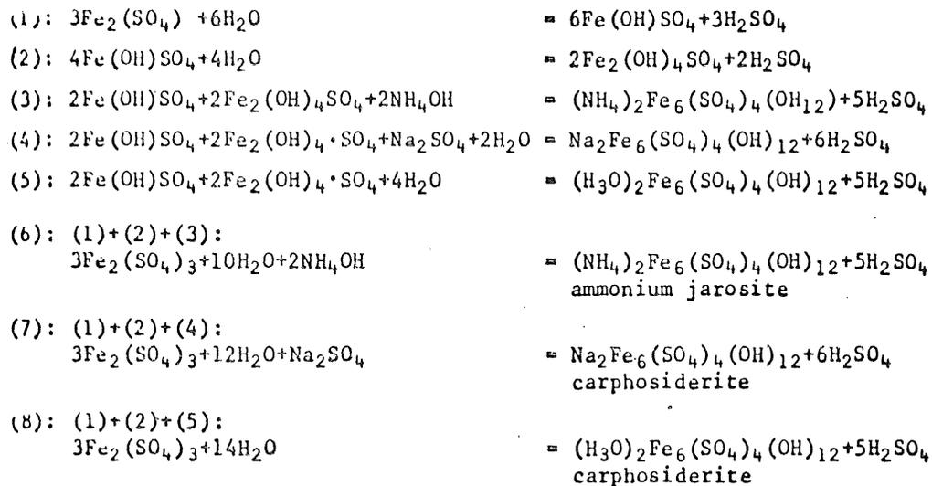
Table 16. Hydrolysis reactions of ferric sulfate.<sup>114</sup>
