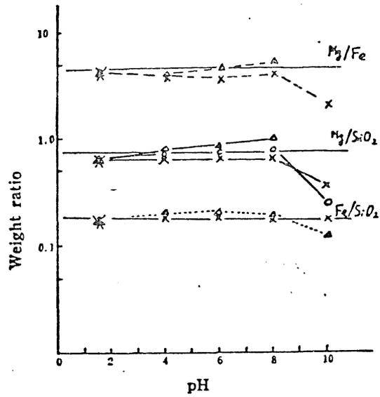
Fig 49. Weight ratios among silica, iron and magnesium dissolved from olivine 149
