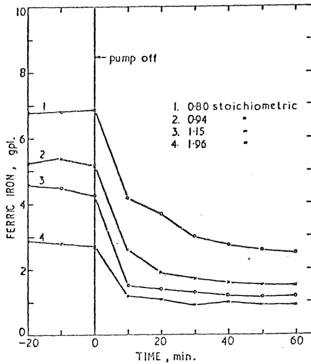
Fig 34 Effect of ammonia additions on iron concentration at 180°C. 106
