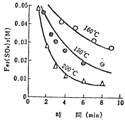
Fig. 38. Rate of  $Fe^{+3}$  hydrolysis 113
