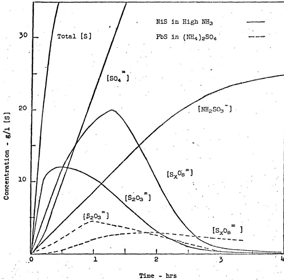
Figure 44. Sulphur Oxidation During An Oxidizing Pressure Leach 10
