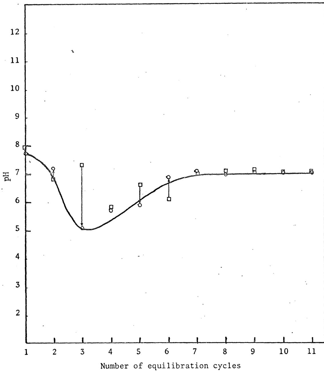
Fig. 51. Equilibration curve for ammonia leach residue
