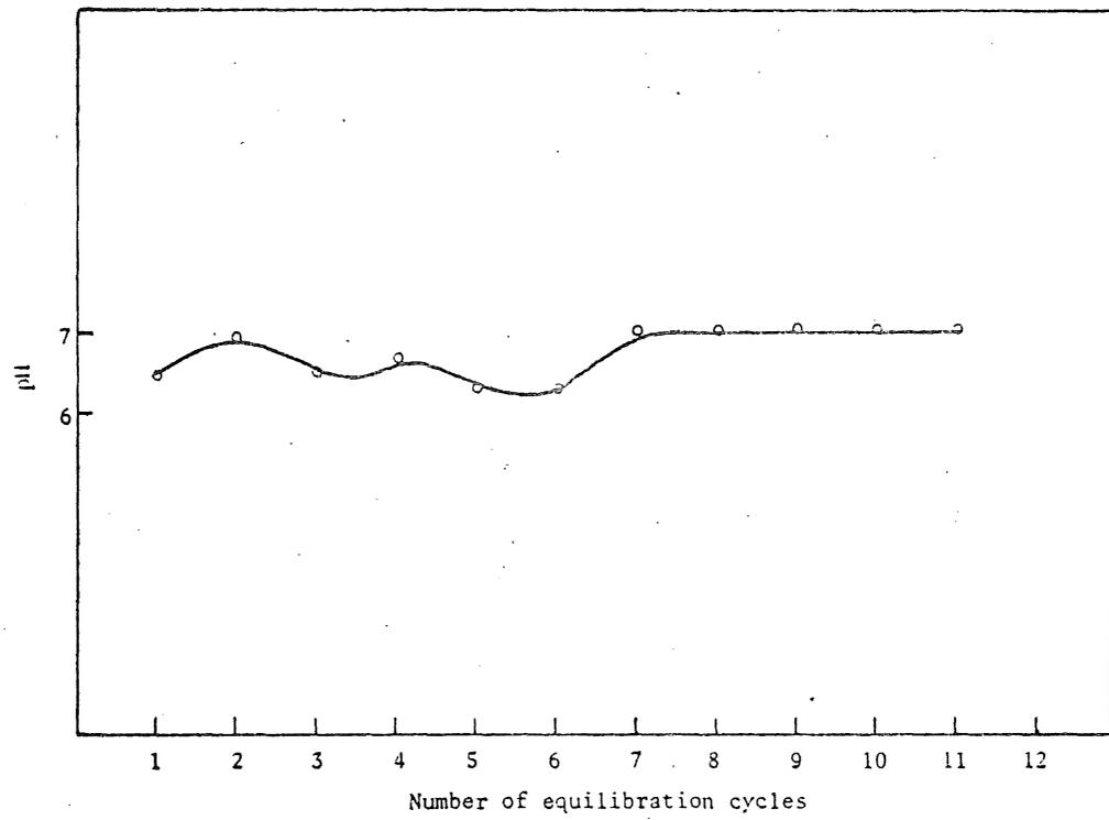
Fig. 58. Equilibration curve for Ferric oxide
