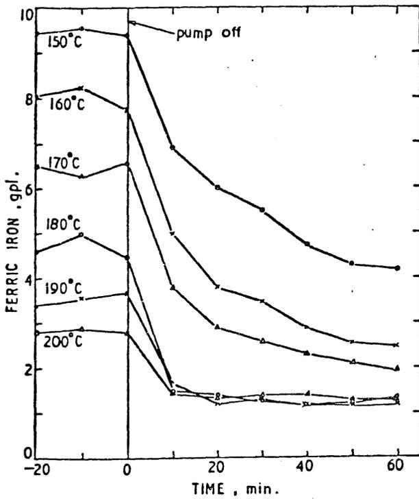
Fig 39 Effect of temperature on iron concentration with stoichiometric addition of ammonia. 106
