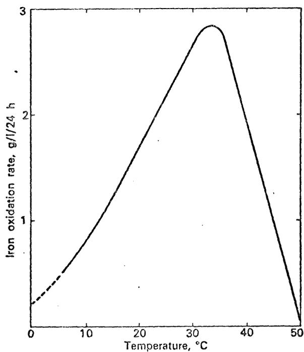
Fig. 20. Effect of temperature on rate of iron oxidation by bacteria. <sup>34</sup>
