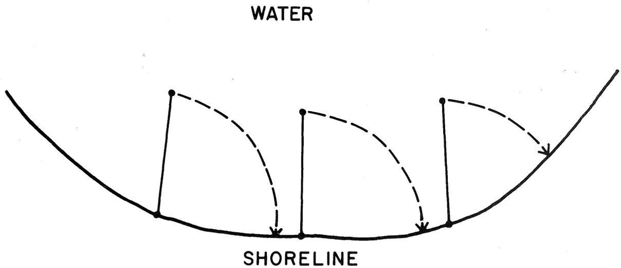
1. Perpendicular to shore line with one braille fixed on the shore and other 100 ft. into lake.
