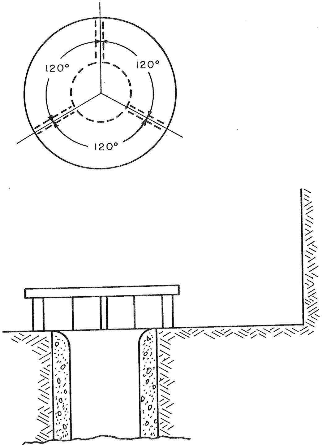
Fig. 8. Covered intake type vortex suppressor (Blaisdell [2]; Humphreys et al. [17]).
