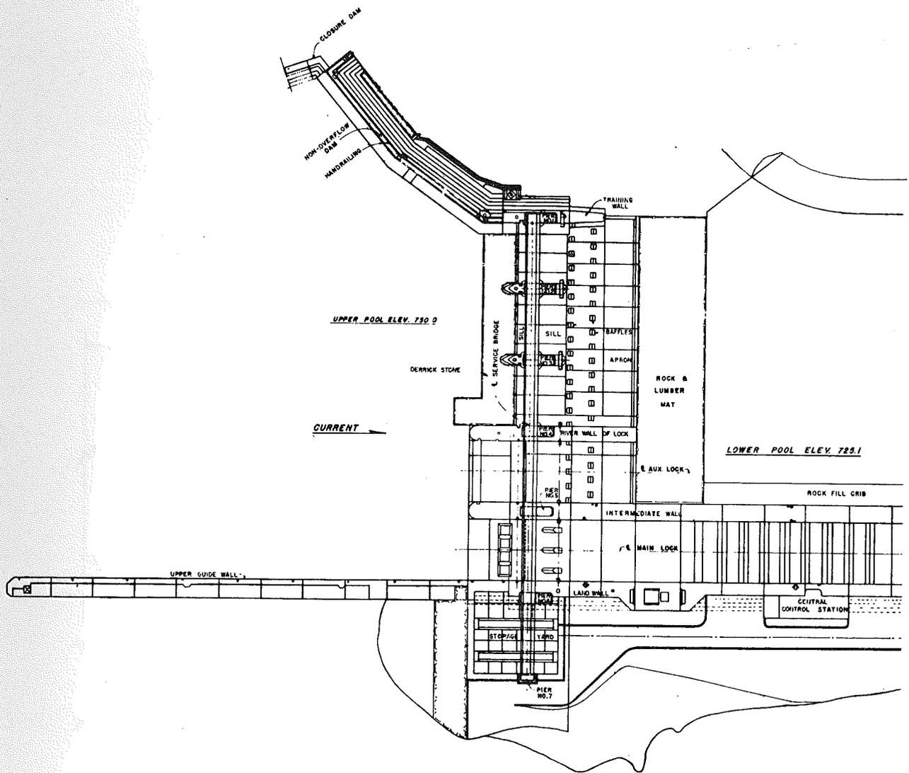
Fig. 9. Plan of the Lower St. Anthony Falls Lock and Dam [1].
