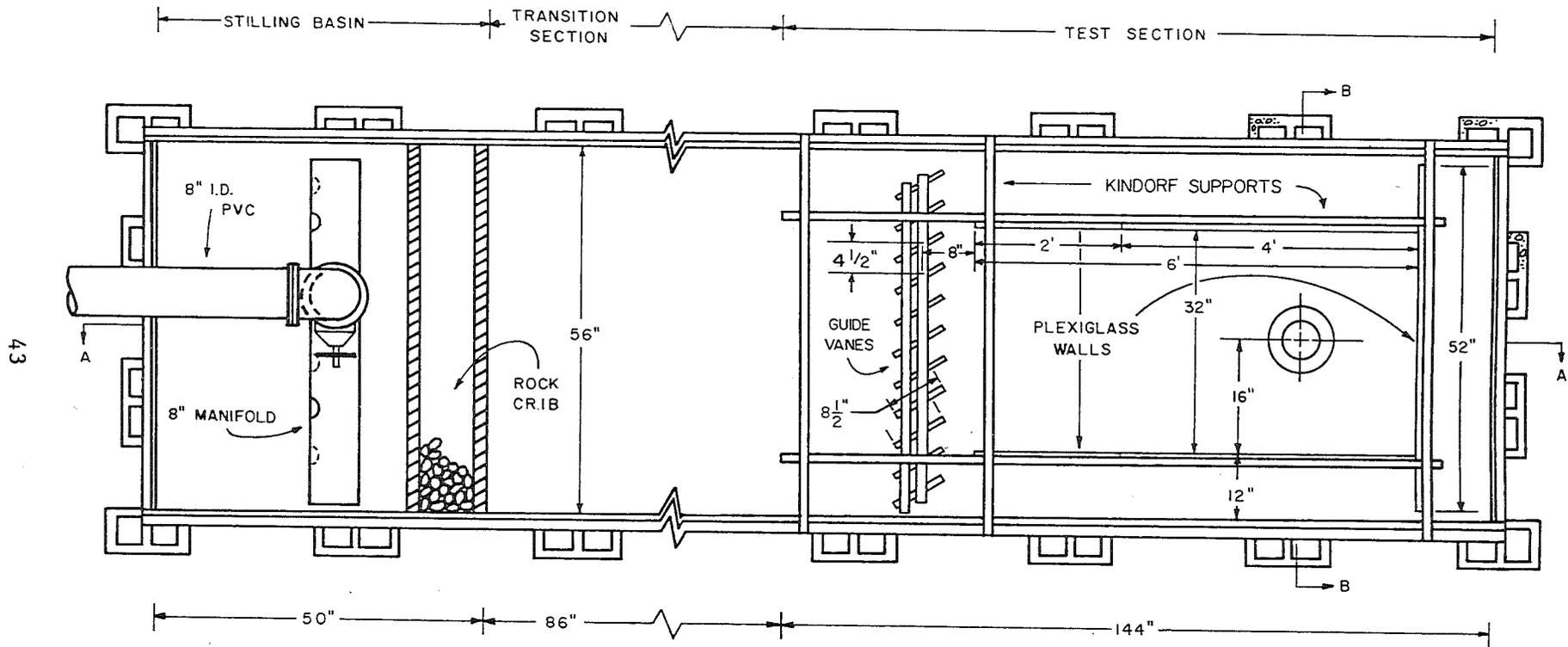
Fig. 20. Plan view of the experimental test facility.
