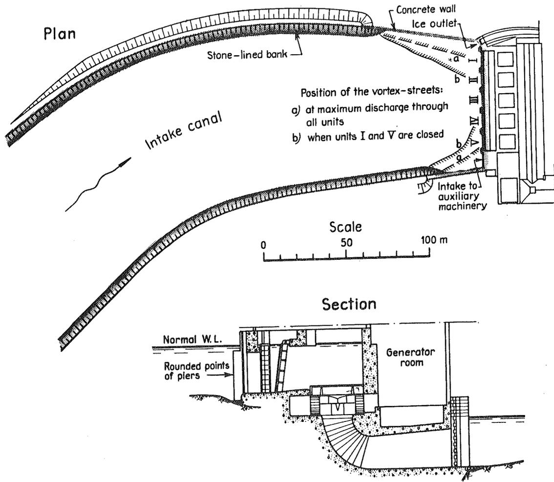
Fig. 14. Untra Power Plant plan and section, taken from Rahm [3].
