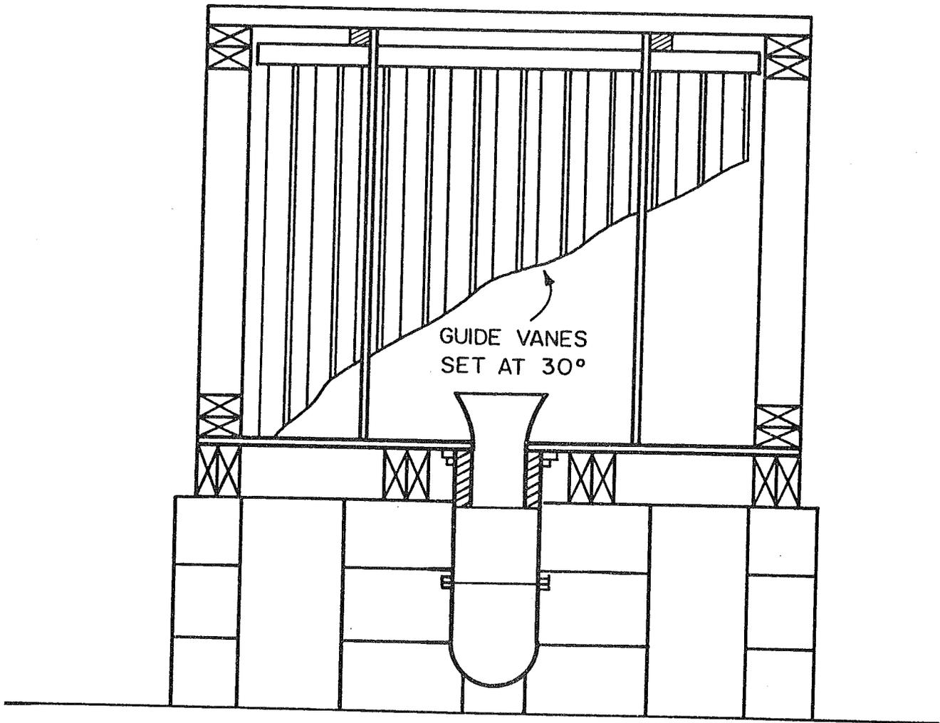
Fig. 22. Section view through the vertical bellmouth intake of the experimental test facility.
