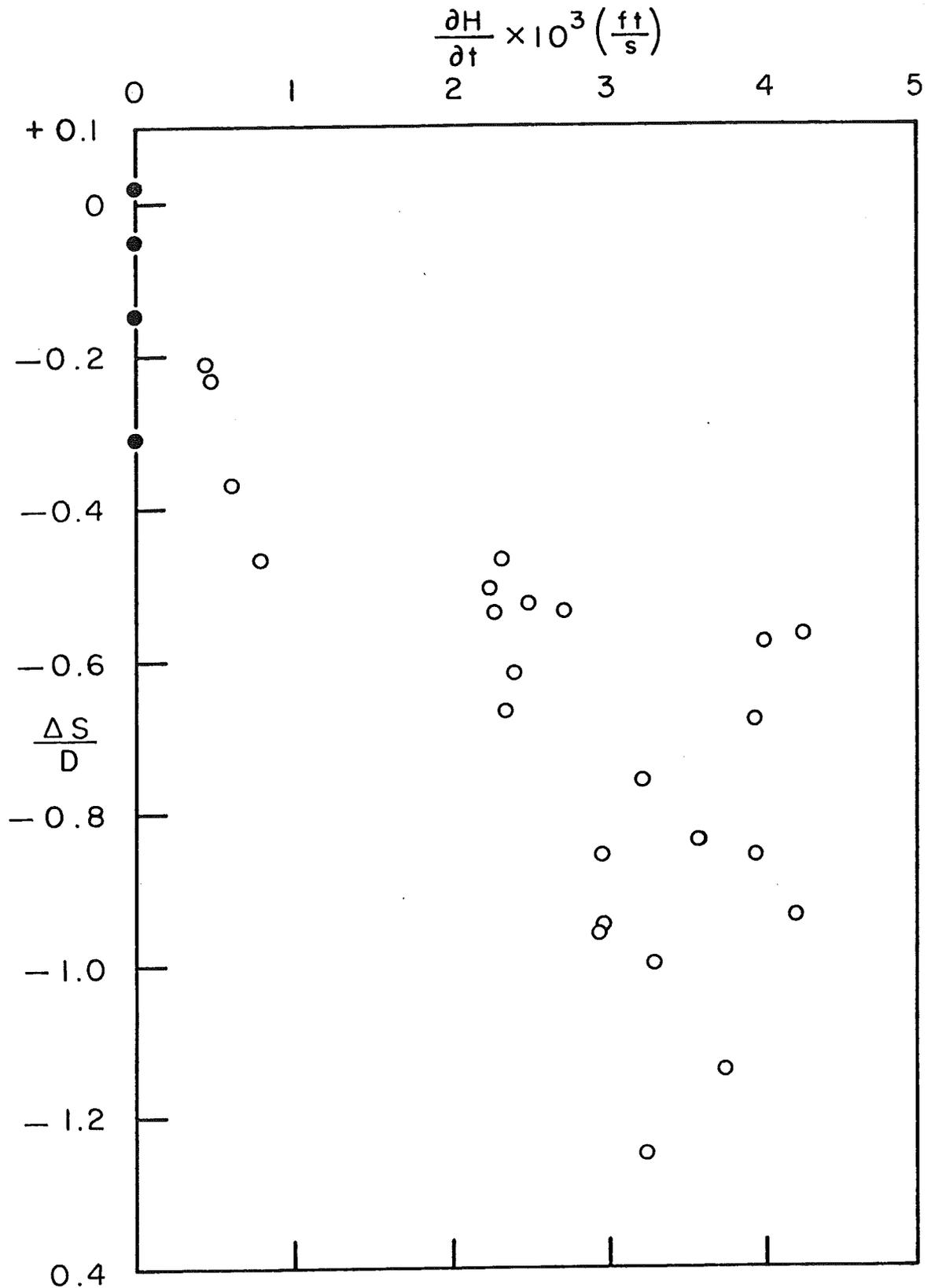
Fig. 38. Difference between actual measurements and envelope curve values of  $S/D$  versus rate of change of water surface elevation for Type 6 vortices. Open symbols - "on the run" measurements. Shaded symbols - steady water surface elevation.
