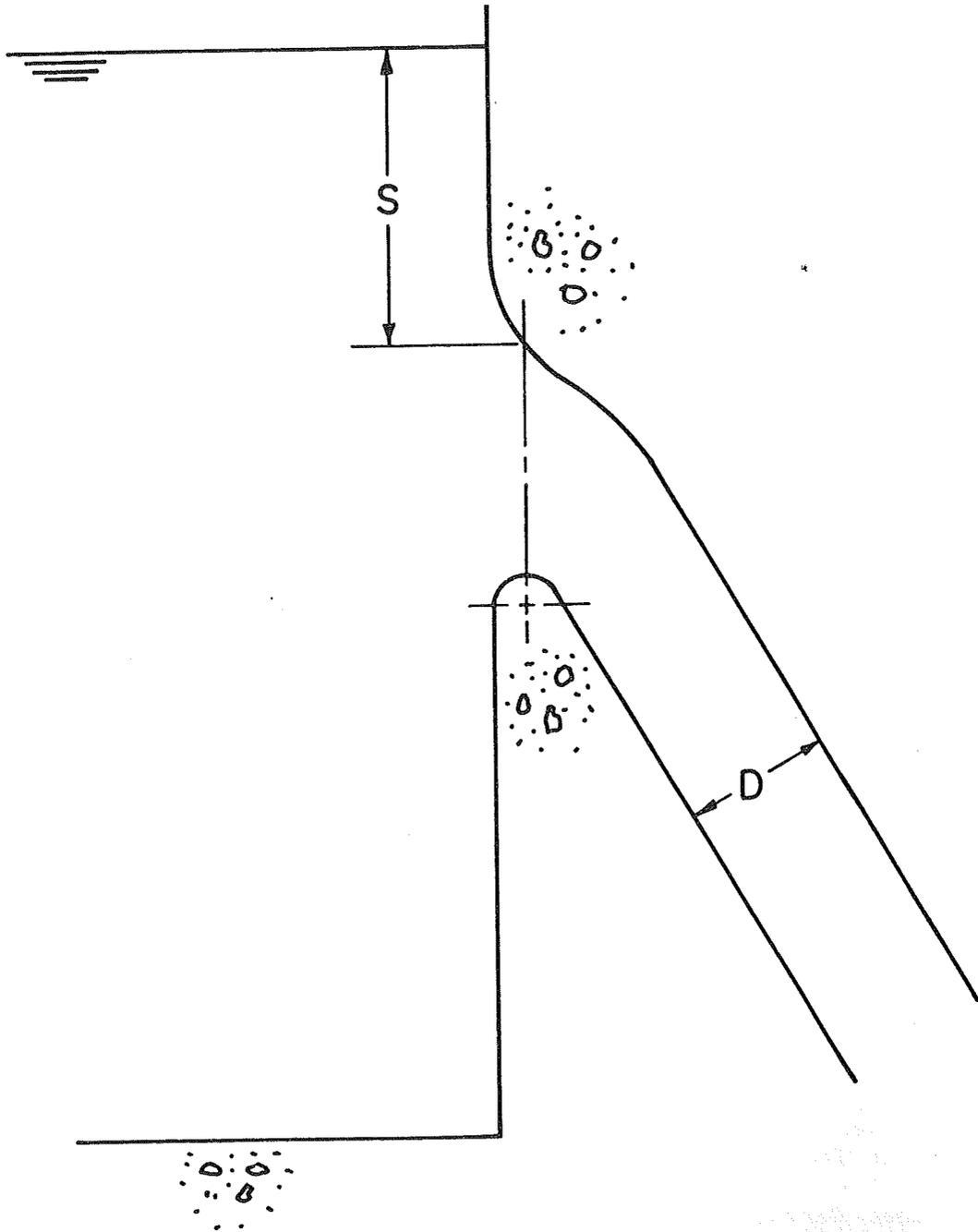
Fig. 18. Definition sketch used to describe submergence,  $S$ , and diameter,  $D$ , of a horizontal intake.
