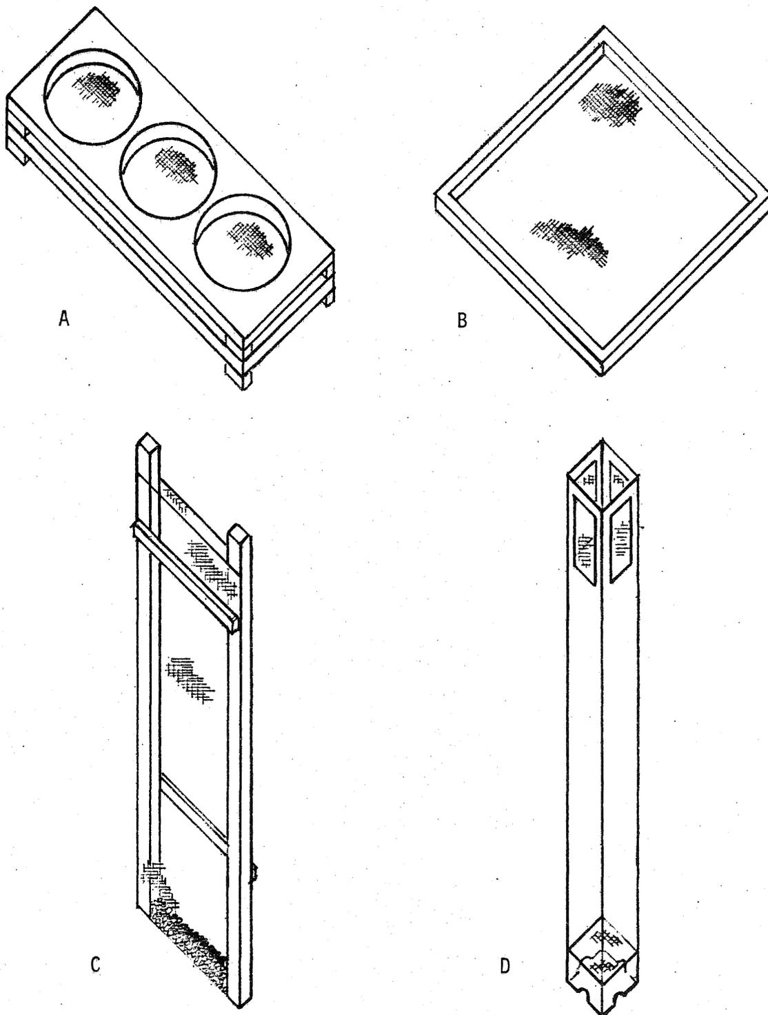
Fig. 1. Egg containers used in experimental incubation of fish eggs. (A), (B) screen-bottom trays, (C) vertical screened container, (D) incubation tube.
