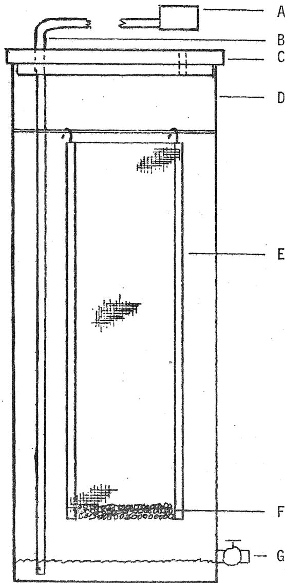
Fig. 2 System for experimental incubation of fish eggs in water-saturated air. (A) air pump, (B) air line, (C) removable top, (D) polyethylene tank, (E) egg container, (F) gravel, (G) water drain outlet.
