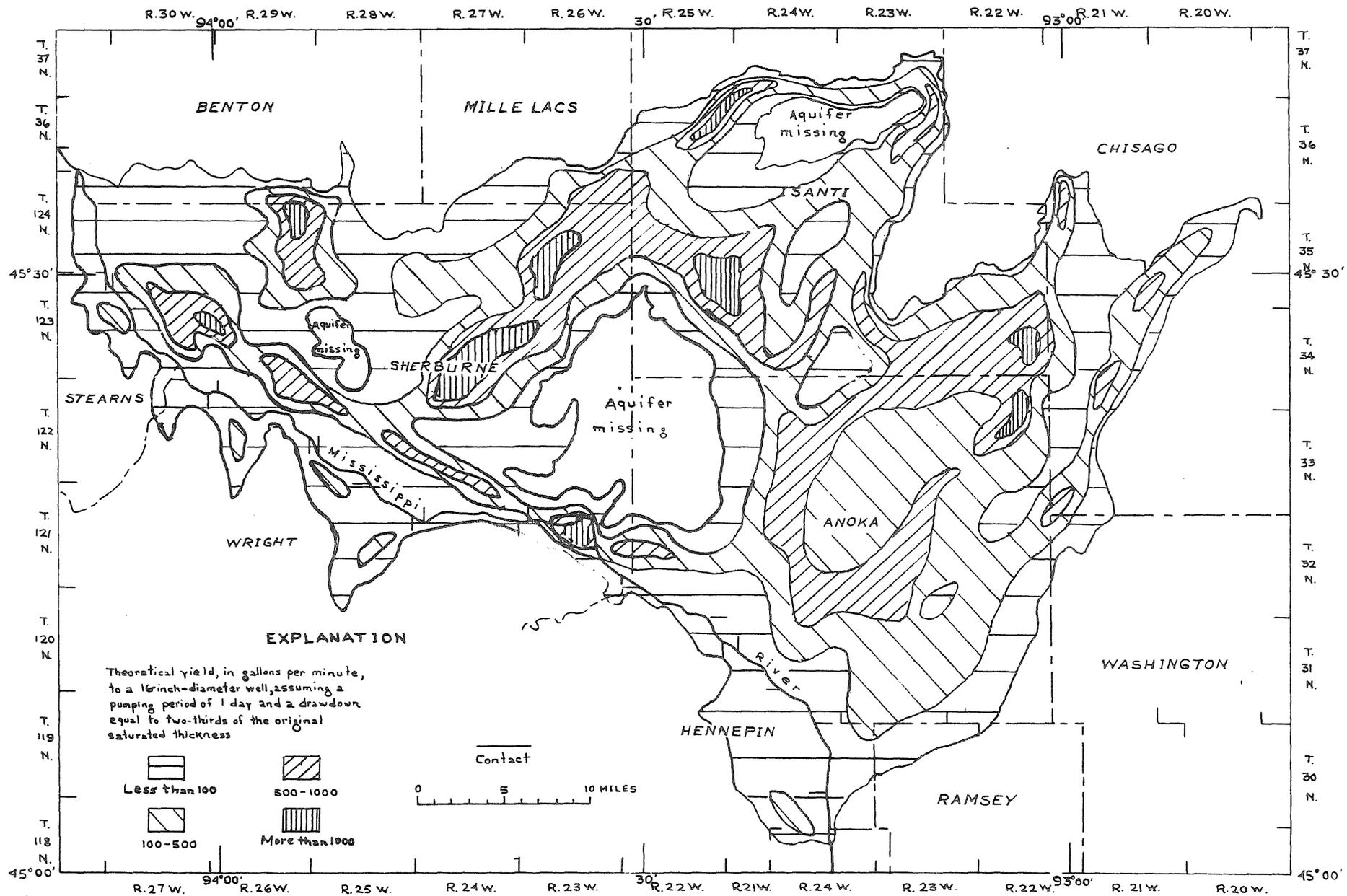
Figure 6.--Theoretical yields to a well completed in the Anoka sand-plain aquifer.
