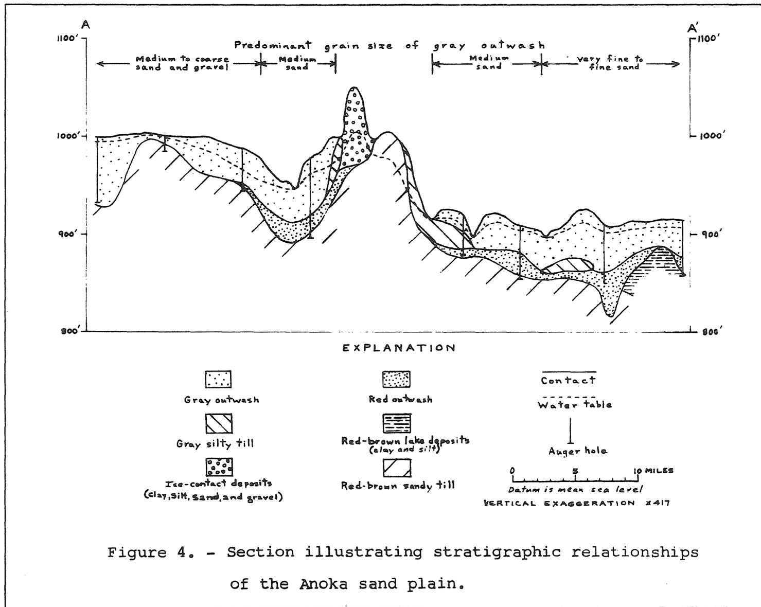
Figure 4. - Section illustrating stratigraphic relationships of the Anoka sand plain.
