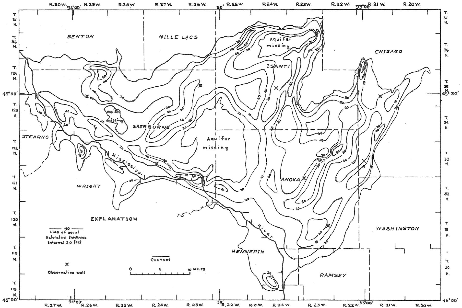
Figure 5. - Saturated thickness of the Anoka sand-plain aquifer.
