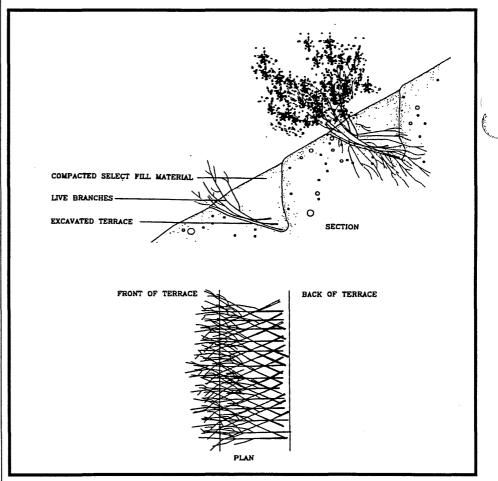
Figure 8: Schematic diagram of an established, growing cut slope brush layer installation, showing alternating layers of live cut brush placed on narrow benches or terraces excavated in the slope. From *Biotechnical and Soil Bioengineering Slope Stabilization, A Practical Guide for Erosion Control*, by Donald H. Gray and Robbin B. Sotir, John Wiley & Sons, 1996. Reprinted by permission of John Wiley & Sons, Inc.
