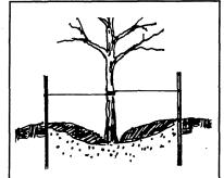
Stake larger trees with two metal stakes, 4-ply hoses and #14 wire for guying. Spread 4-6 inches of mulch; keep mulch away from trunk.
