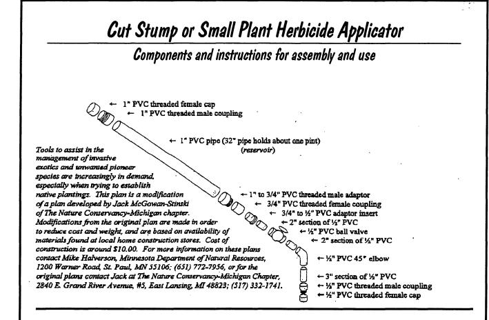
Assembly Instructions: Cement all non-threaded parts together using PVC pipe cement. To prevent leakage, be sure to use Tetion plumbing tape on all of the threaded parts. Before attaching the ½" PVC threaded female cap, drill two 1/16" drip holes near the center of the cap. More holes can be added later if you feel additional flow is needed.
