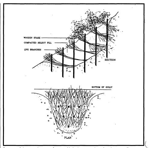
**Figure 5: Schematic diagram of an established, growing branchpacking installation.** From *Biotechnical and Soil Bioengineering Slope Stabilization, A Practical Guide for Erosion Control,* by Donald H. Gray and Robbin B. Sotir, John Wiley & Sons, 1996. Reprinted by permission of John Wiley & Sons, Inc.
