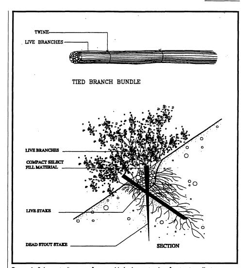
**Figure 6: Schematic diagram of an established, growing live fascine installation,** showing live fascine bundles (above) and method of placement in a slope (below). From *Biotechnical and Soil Bioengineering Slope Stabilization, A Practical Guide for Erosion Control,* by Donald H. Gray and Robbin B. Sotir, John Wiley & Sons, 1996. Reprinted by permission of John Wiley & Sons, Inc.
