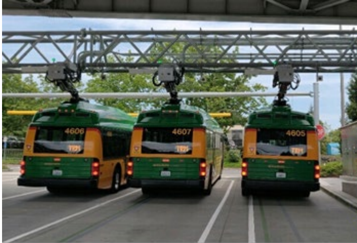
Figure 26: King County Overhead Gantry Charging System
