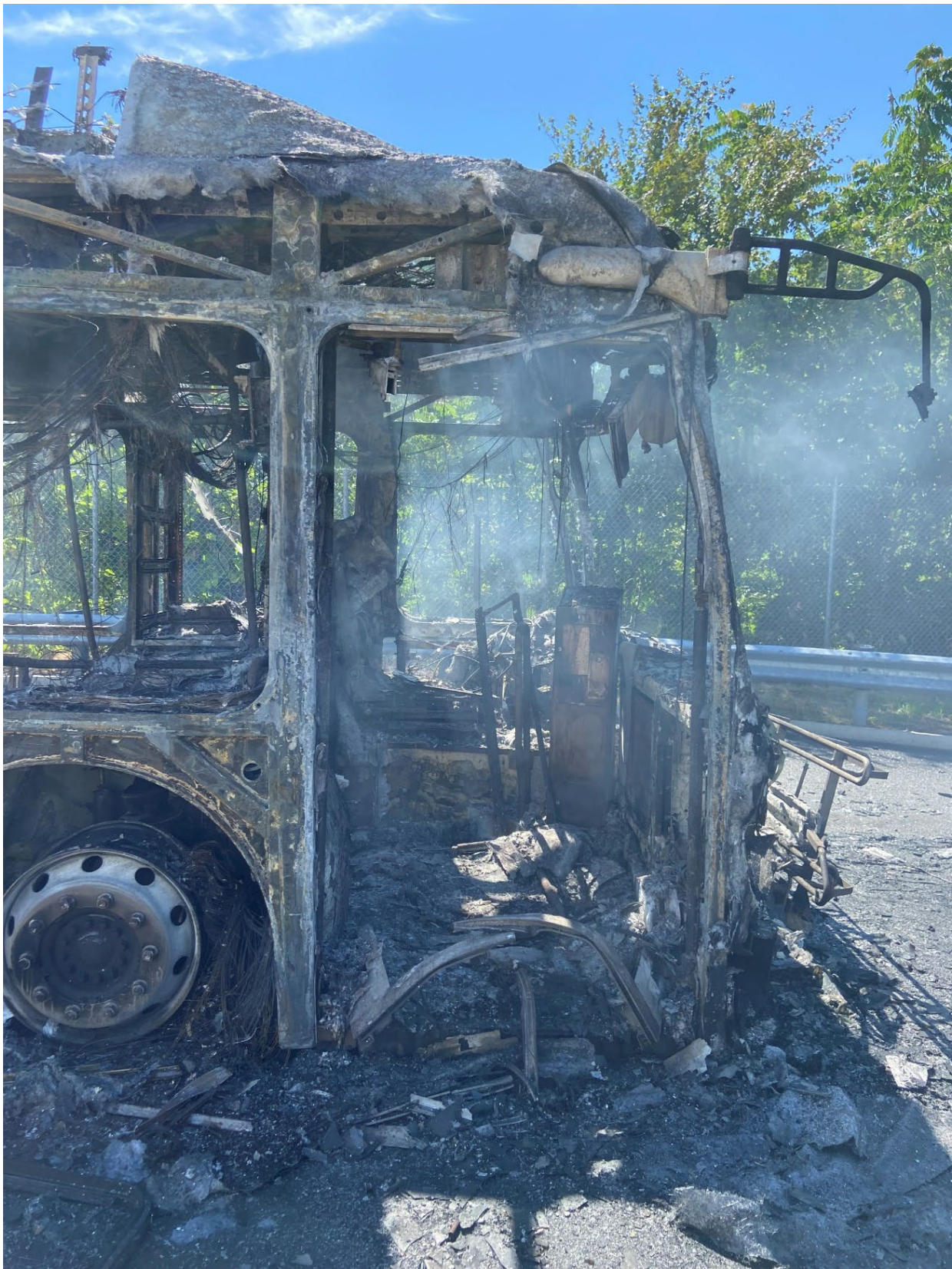
Figure 65: Bus after a 2022 BEB fire in Hamden, Connecticut 266
