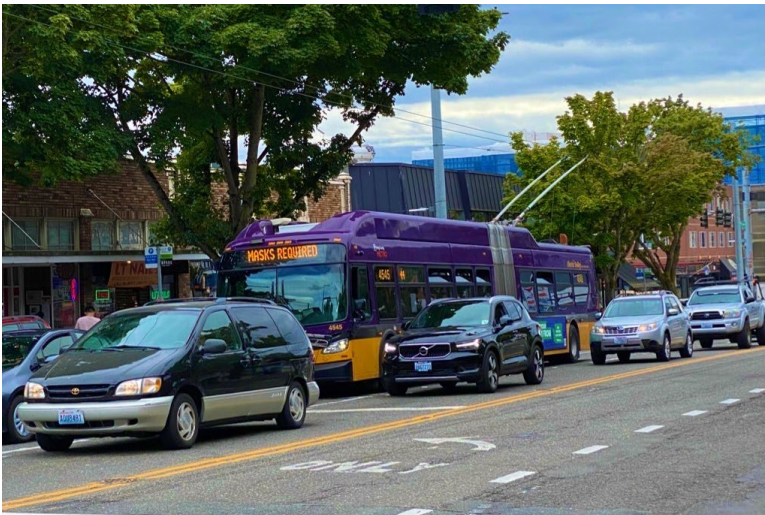
Figure 9: Trolleybus in Operation with Two Trolley Poles in Seattle, Washington
