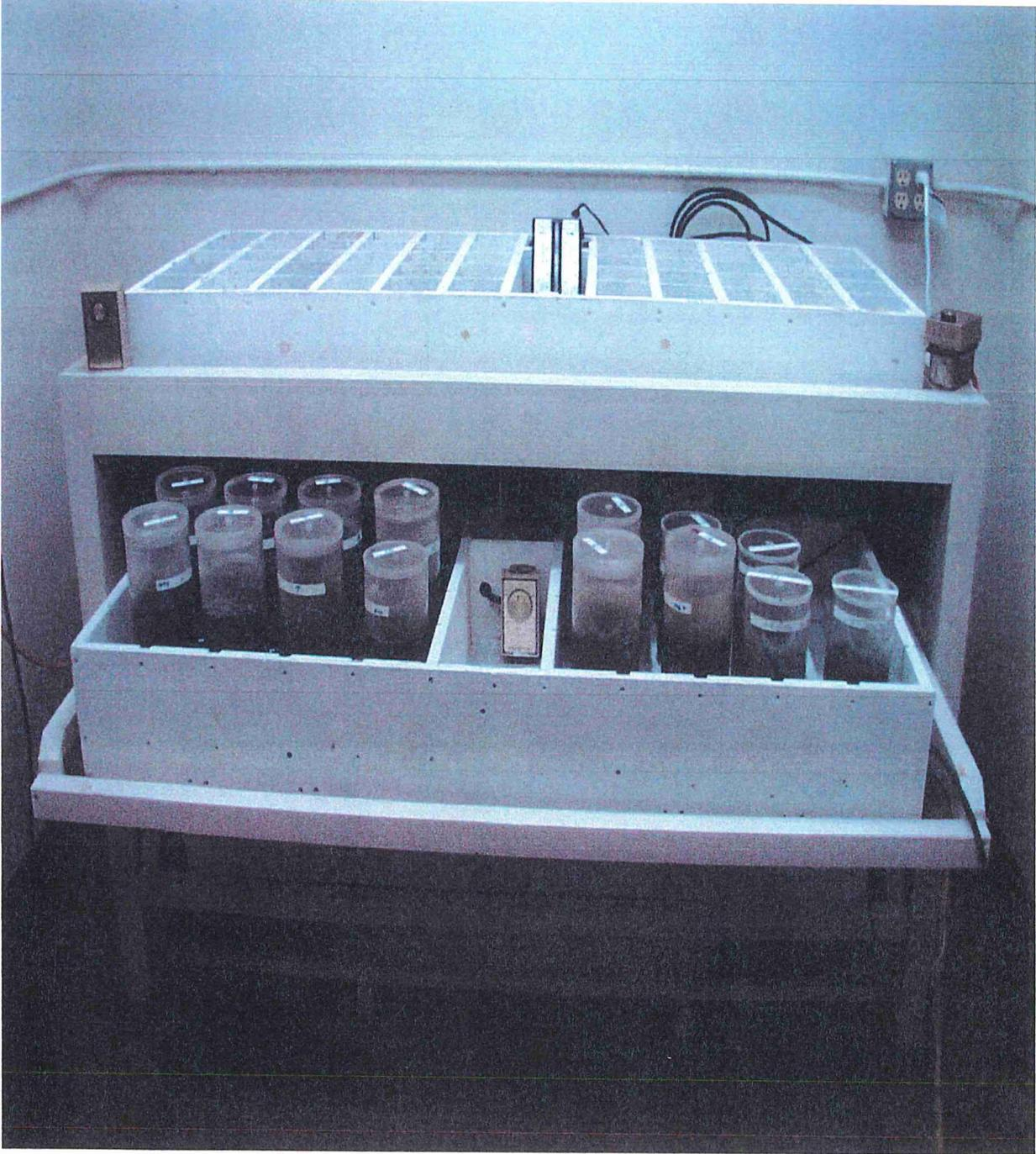
Figure 5. KB-SEA™ reactors, side view. Distribution of material in the KEECO cells reactors immediately after application. Since this was a slurry you could see the distribution within the reactor. Left to right, 5%, 3%, 1%.
