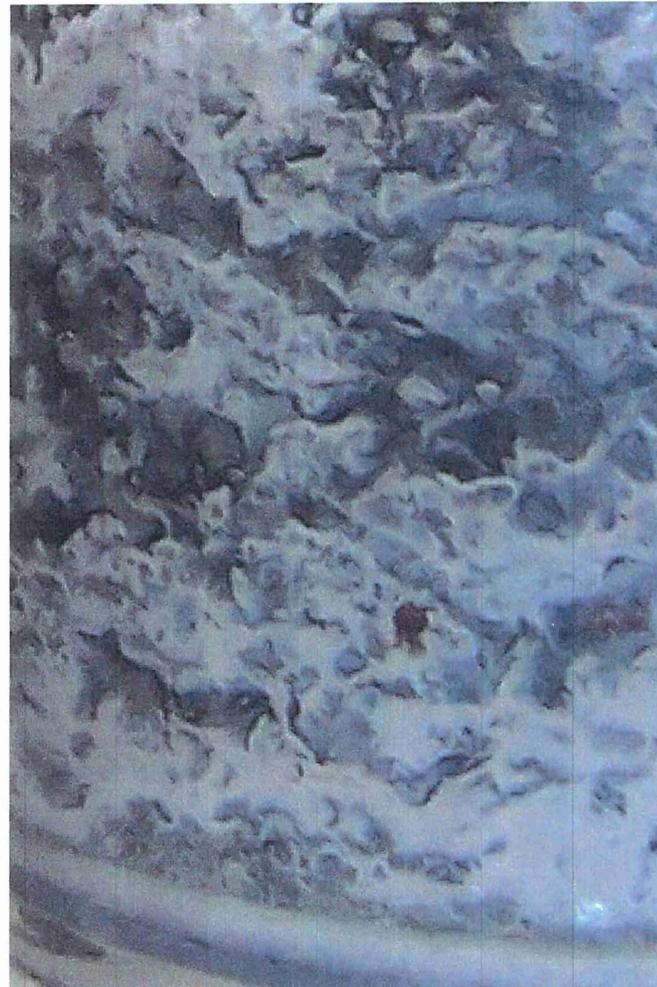
Figure 37. Material treated with 3% KB-SEA™. Images show oxidation has occurred despite visible coating.
