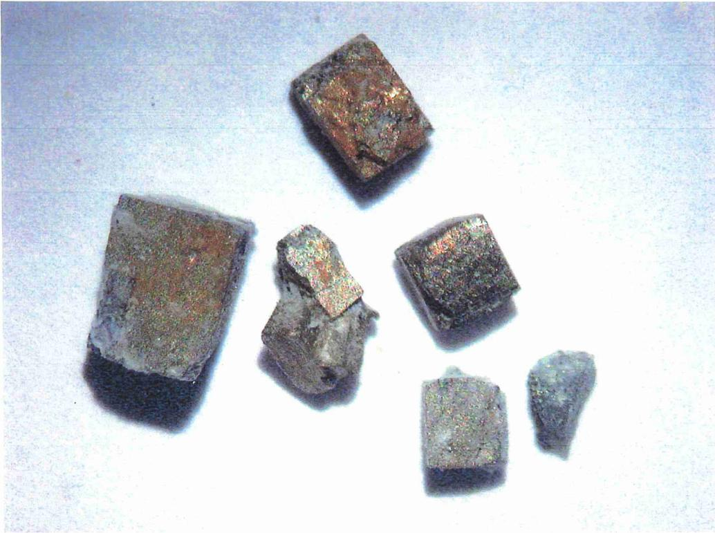
Figure 13. Pyrite cubes from unleached KEECO reactor.
