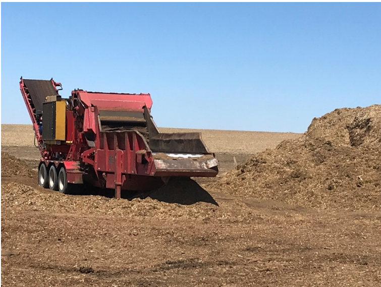
Figure 2: Horizontal grinder used for composting carcasses
