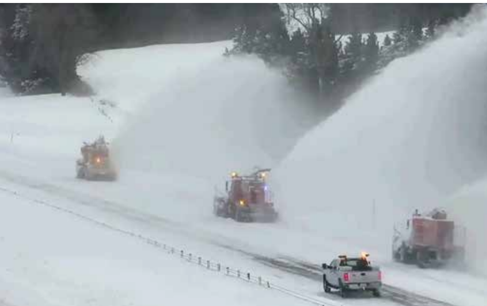
Three snow blowers work together to clear drifts along I-35 near Ellendale
