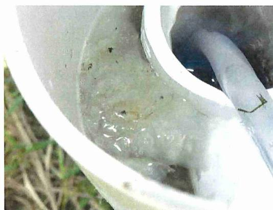
*Photos of biofilm clogging woodchip bioreactors. a) biofilm inside the woodchip sampling port. b) biofilm accumulation at the inlet pipe and acetate injection site.*
