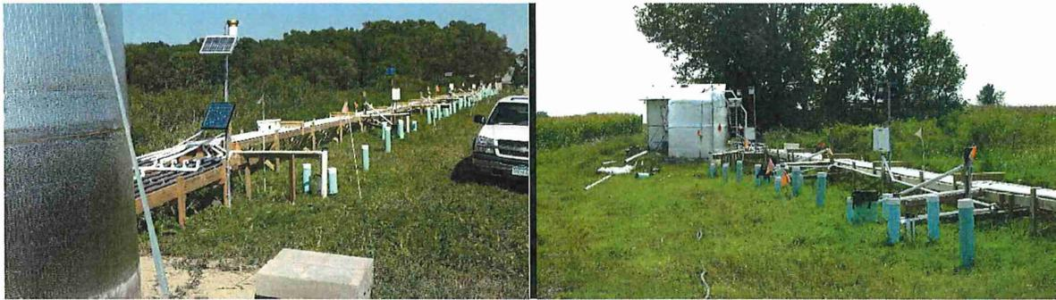
Fig. 3. Photos of the supply tank and the tile-water distribution system to each bioreactor bed.
