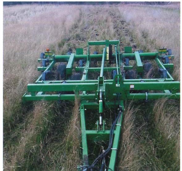
*Chisel plow used to disturb sod-bound intermediate wheatgrass field in an effort to restore grain yield.*
