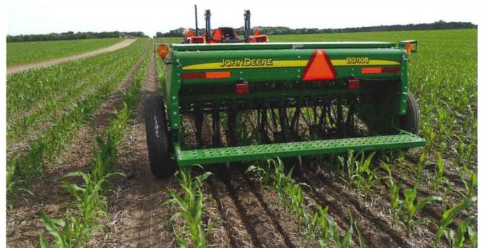
*We used an 8' grain drill with four planting units to inter-seed the cover crops in 2016.*
