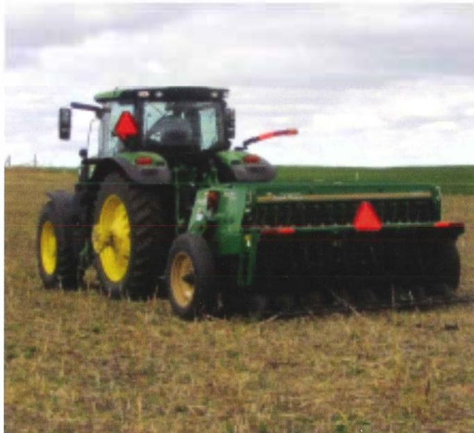
We used a no-till drill to plant the intermediate wheatgrass into a well-grazed plot.
