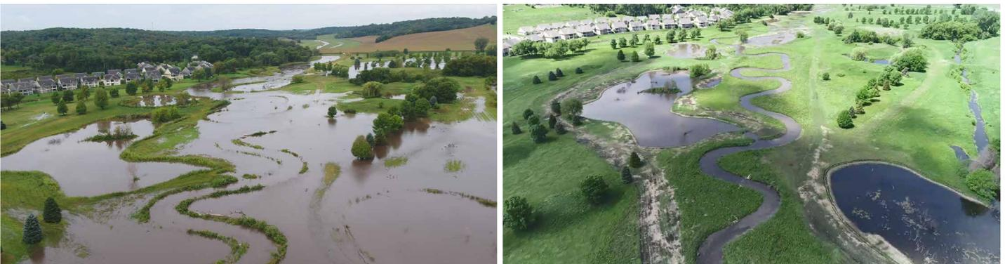
Figure 1. Restored stretch of Cascade Creek in Olmsted County. **Left:** During September 2018 flood; water spreading out across the floodplain and into constructed wetlands. **Right:** Waters receded after the flood. The main stream channel withstood the test and continues to perform well.
