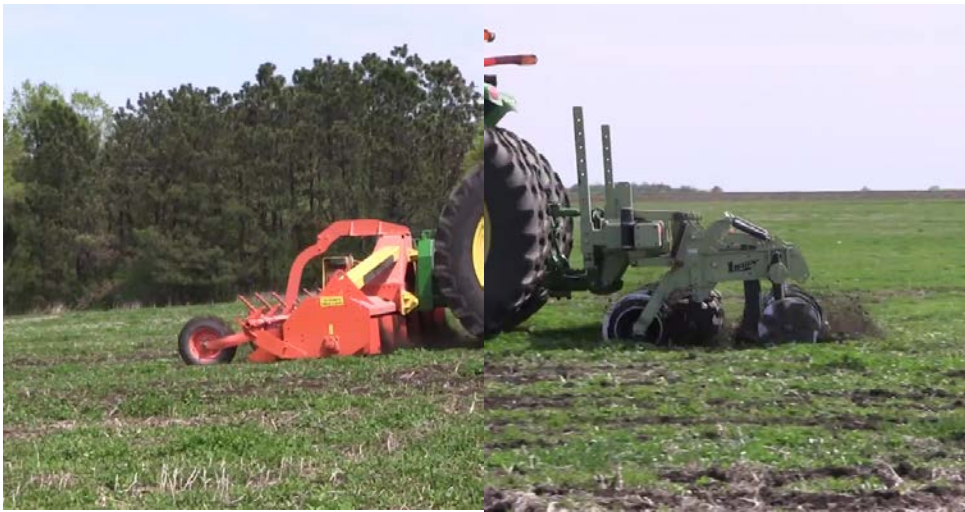
Left: Rotary Zone Till implement (ZT), Right: Shank Till (ST) implement. Double Till (DT) treatments combined ZT and ST.
