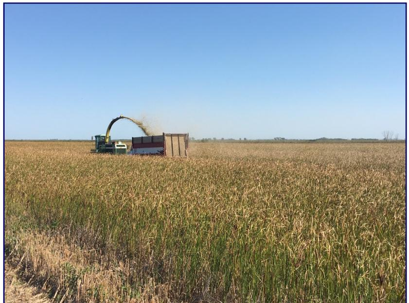
*Photo: Cattail biomass harvesting conducted in 2016 using conventional forage chopping equipment. Harvested biomass is then land applied as an agricultural soil amendment*
