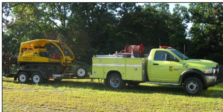
Type 6 engine towing J-5 tracked vehicle
