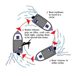
If you notice that it takes extra pressure on the steering wheel or handle, have your boat serviced immediately. On some smaller outboards, repair may be as simple as tightening a bolt.
