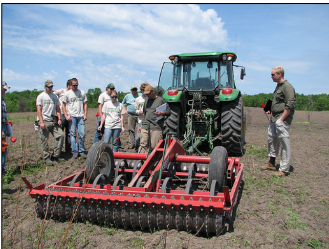
Using a cultipacker to ensure good seed to soil contact
