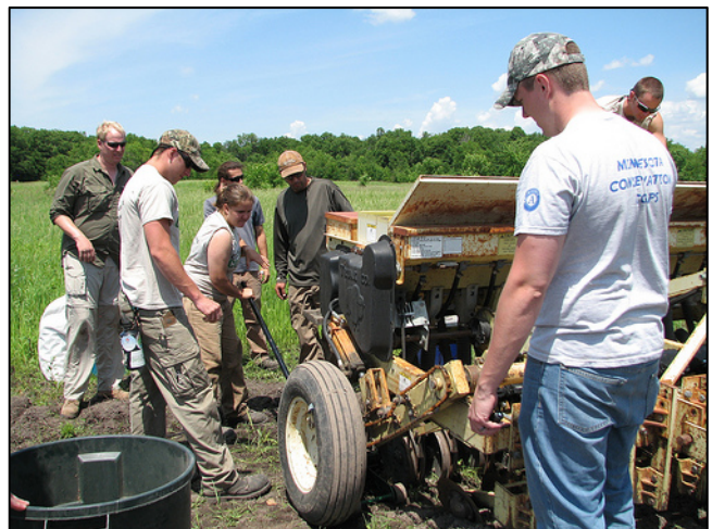
Jacking up the seed drill in preparation for calibrating it
