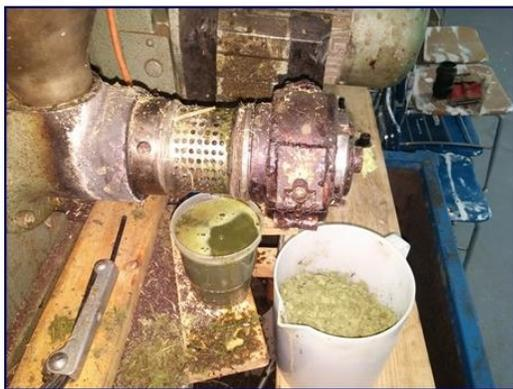
*Separation of liquid from plant solids in growing cattail at the University of Minnesota, Crookston to analyze agriculture related nutrient utilization potential.*
