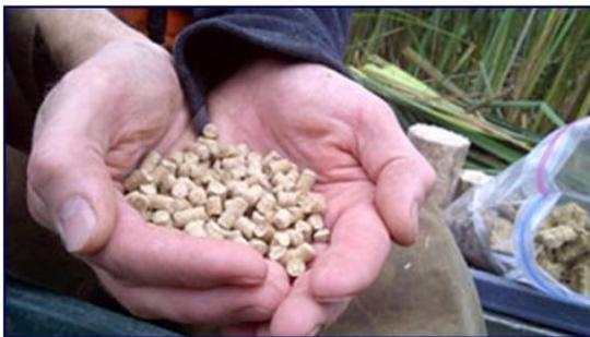
**LEFT:** Pelletized cattails have burning quality similar to wood pellets and high absorption capacity creating a product suited well to hazardous spill absorption.
