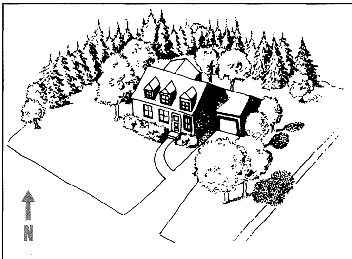
Figure 5. A windbreak on the west and north of the building and shade trees on the east and west of the building significantly reduce the cost of heating and cooling.
