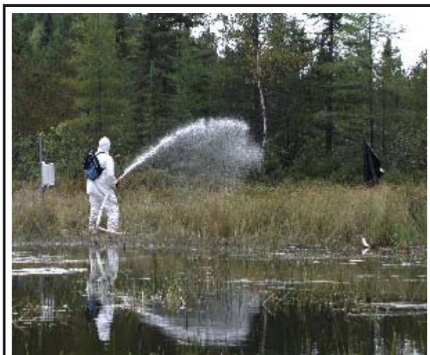
Applying a solution of water and a stable isotope of mercury ( ^{202}\text{Hg} ) on the shores of a lake in the Experimental Lake Area (ELA) in Ontario, Canada. An international team of scientists tracked the applied mercury isotope to study the movement of mercury from the watershed into the lake and fish. ( Larger version )
