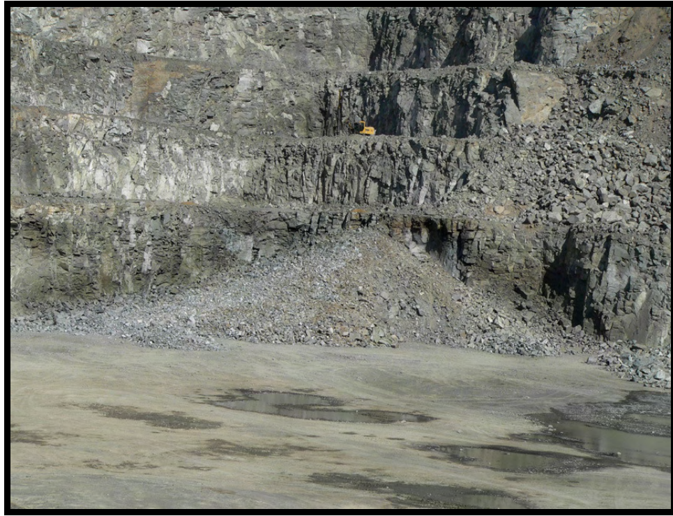
Figure A4.4 – Rock left after a blast
