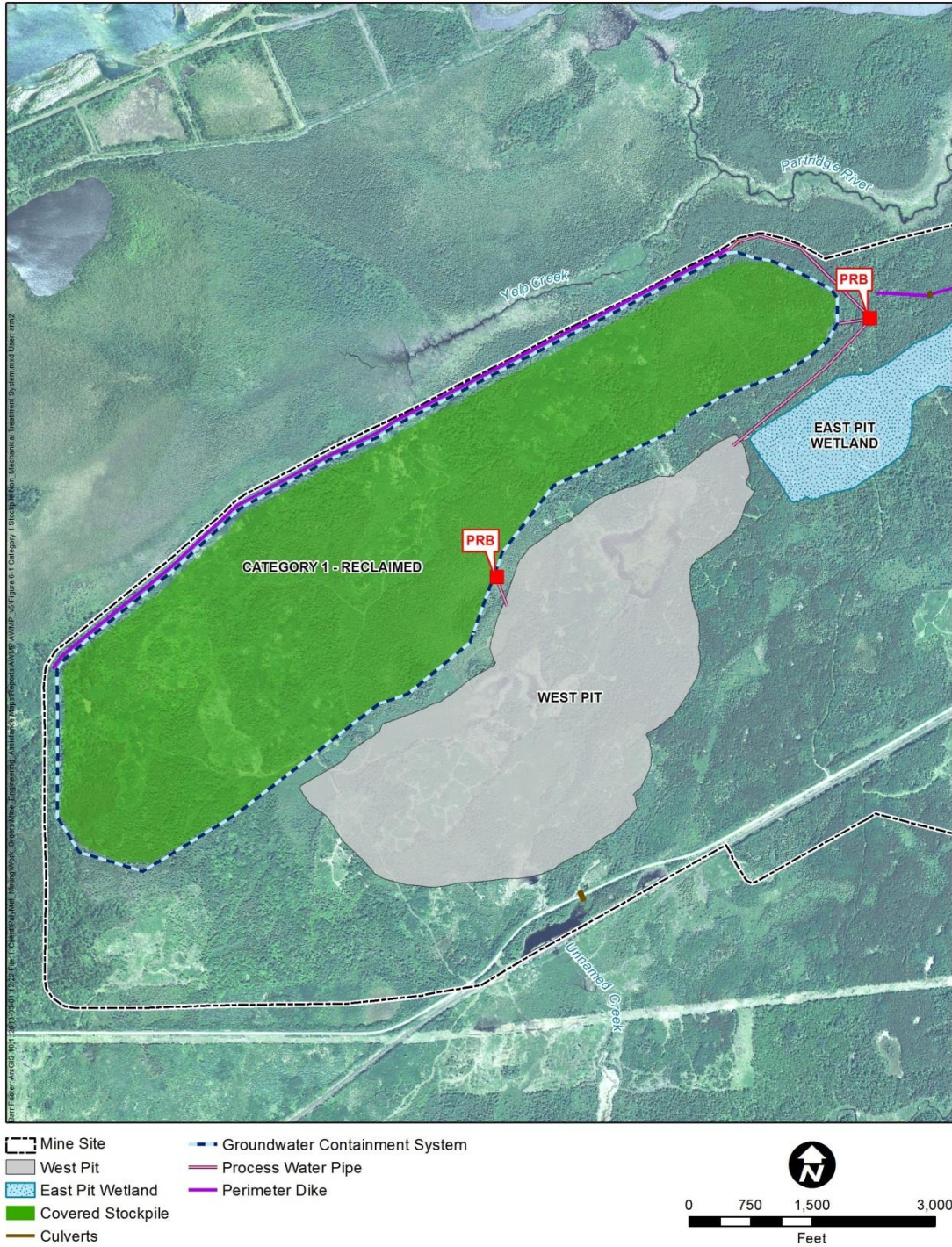
Figure 6-1 Conceptual Plan View: Category 1 Waste Rock Stockpile Non-Mechanical Treatment System
