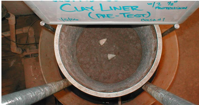
Figure 1 – Clay liner with rock protrusions, pre-test.
