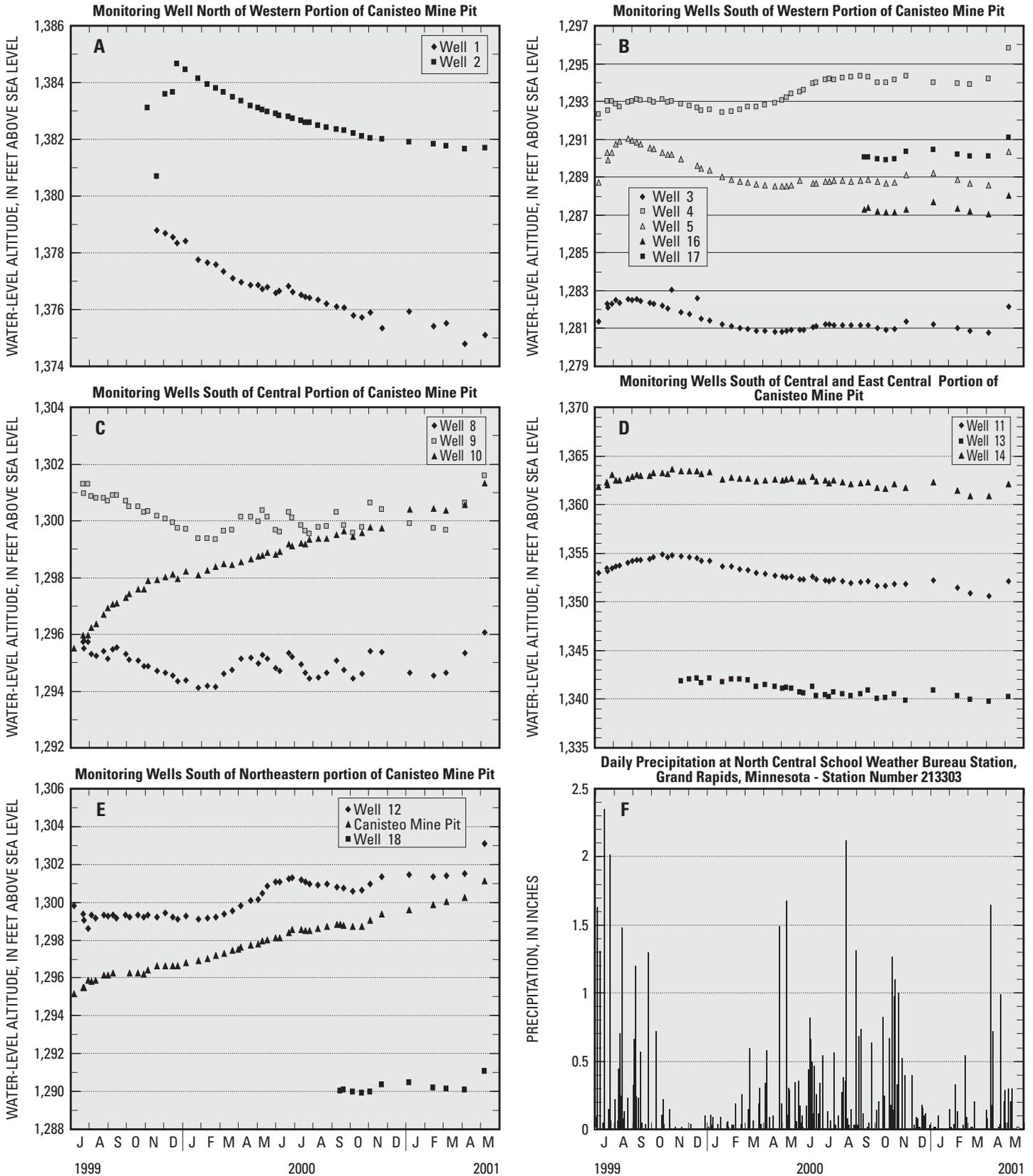
**Figure 5.** Water-level altitudes in monitoring wells surrounding the Canisteo Mine Pit, Bovey, Minnesota, water-level altitudes in the Canisteo Mine Pit, and daily precipitation at North Central School Weather Bureau Station, Grand Rapids, Minnesota - Station Number 213303, July 1999-May 2001 (Well numbers shown in figure 3).
