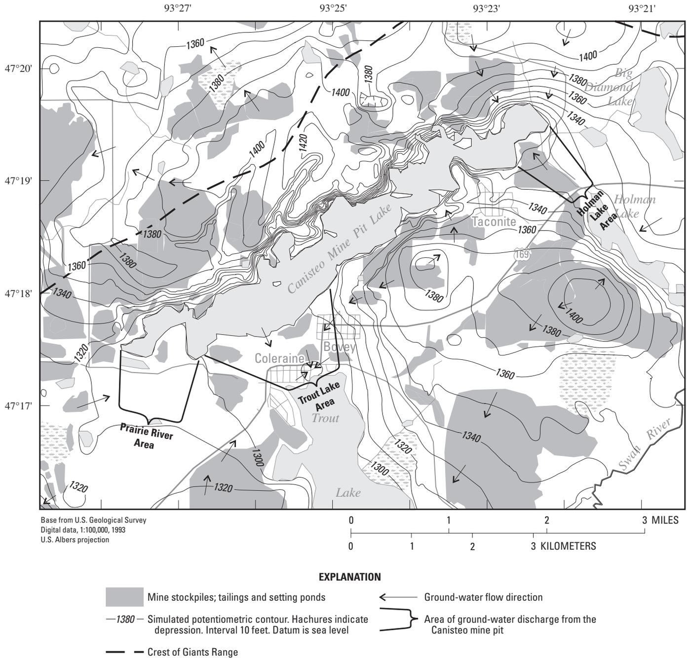
**Figure 7.** Simulated steady-state altitude of potentiometric surface of ground-water flow and ground-water flow direction in the vicinity of the Canisteo Mine Pit, Bovey, Minnesota (Constant pit water-level altitude of 1,300 feet above sea level).
