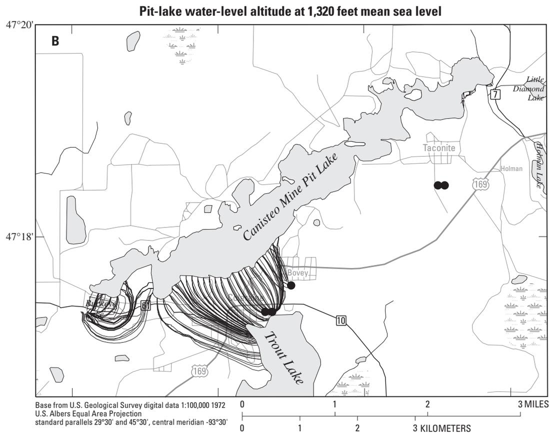
**Figure 8.** MODPATH flow lines for ground-water outflow from Canisteo Mine Pit at pit water-level altitude of: A.) 1,300 and B.) 1,320 feet above mean sea level, Bovey, Minnesota.
