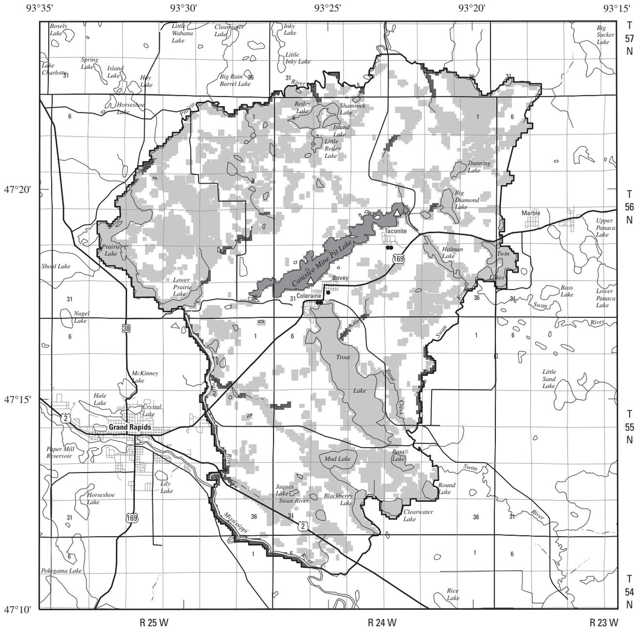
**Figure 4.** Model segmentation for MODFLOW simulation of aquifers surrounding the Canisteo Mine Pit, Bovey, Minnesota.
