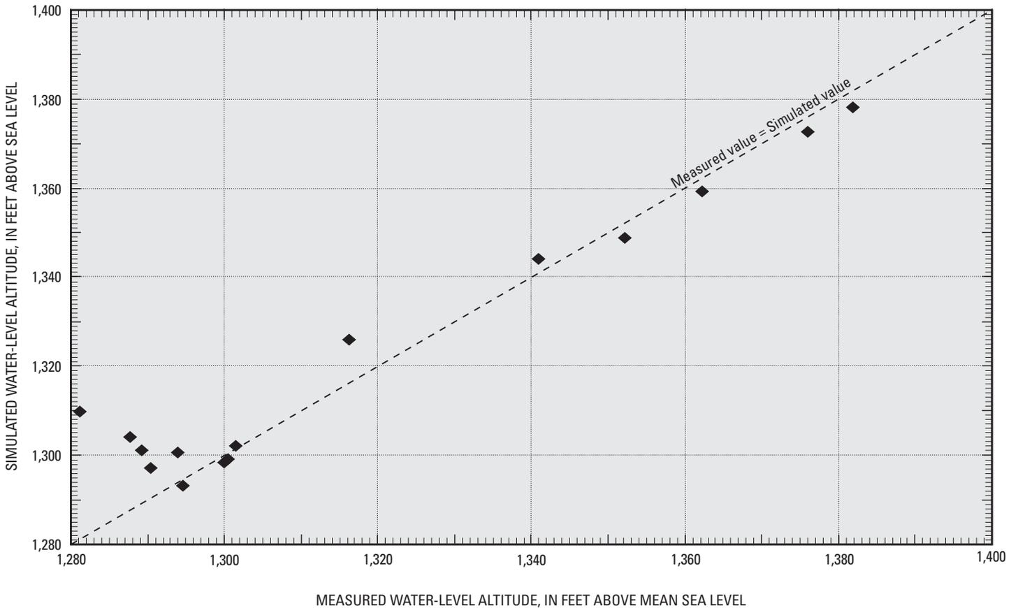
**Figure 6.** Measured versus simulated water-level altitude in monitoring wells at a constant pit water-level altitude of 1,300 feet above sea level (see table 5).
