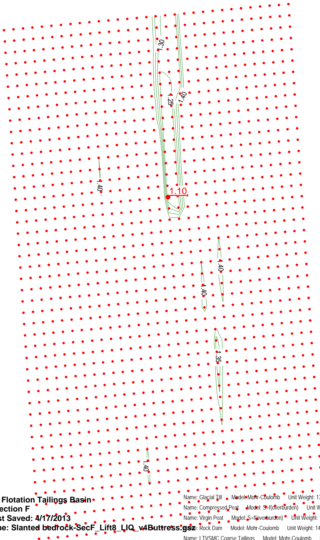
Figure 7. Fully Liquefied Section F - Cell 2W Lift 8: Cutoff Wall - Drainage System Idle (LIQ)
