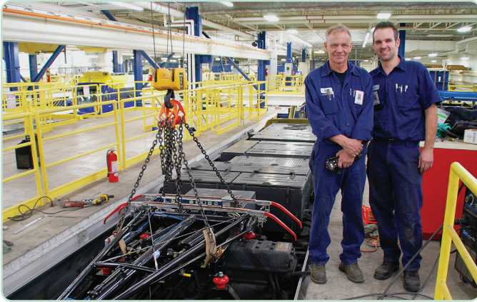
Technicians service the electrical components on the roof of a light rail vehicle at the METRO Blue Line operations and maintenance facility.
