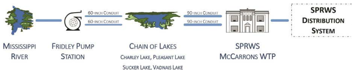
Figure 1. Saint Paul Supply System Schematic
