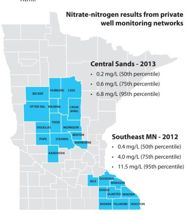
This map shows summary statistics from two private well monitoring networks in Minnesota. The 50th percentile (75th, 95th) is the value below which 50 percent (75%, 95%) of the observed values fall. The health standard for nitrate-nitrogen in drinking water is 10 mg/L.
