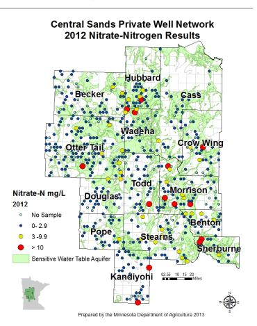
This map shows nitrate-nitrogen analysis results from the Central Sands Private Well Monitoring Network in 2012. The health standard for nitrate-nitrogen in drinking water is 10 mg/L.
