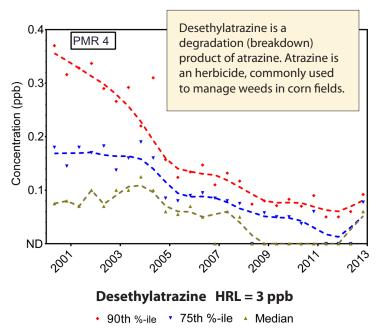
This is an example of results from MDA's monitoring program and displays the trend in desethylatrazine concentration over time. Results are from Pesticide Monitoring Region (PMR) 4, which encompasses a 14-county area in central Minnesota.
