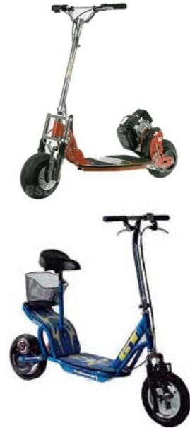
Models are available with either gas and electric motors. Electric models generally have a top speed below 15 miles per hour and a range of up to 20 miles. Ones with gas engines commonly range from 25 to 50 cc (1.5 to 2.5 horsepower) and can have a top speed of over 30 miles per hour.
