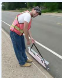
The handheld electromagnetic gauge is a promising tool for non-destructive testing of moisture levels in and beneath pavement layers.
