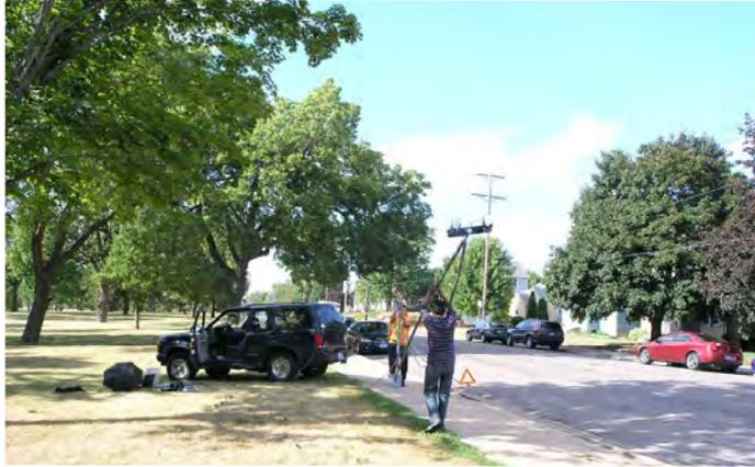
Researchers used a portable camera boom system to gather observational data on vehicle-crosswalk and vehicle-pedestrian interactions at uncontrolled crosswalks in the Twin Cities metropolitan area.
