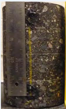
Counties provided 6-inch-diameter wear and nonwear course core samples for the evaluation of dynamic modulus and other properties.
