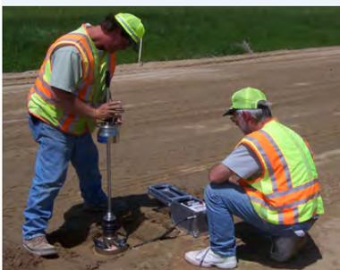
An LWD repeatedly drops a mass on a loading plate in contact with the ground to estimate its stiffness.
