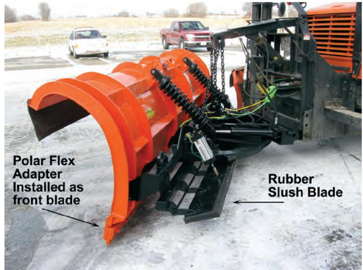
Clear Roads recently funded the development of innovative prototype snowplows capable of tackling a range of winter road conditions using multiple plow blades. For more information, see [www.clearroads.org/multiple-blade-plow-prototypes.html](http://www.clearroads.org/multiple-blade-plow-prototypes.html).
