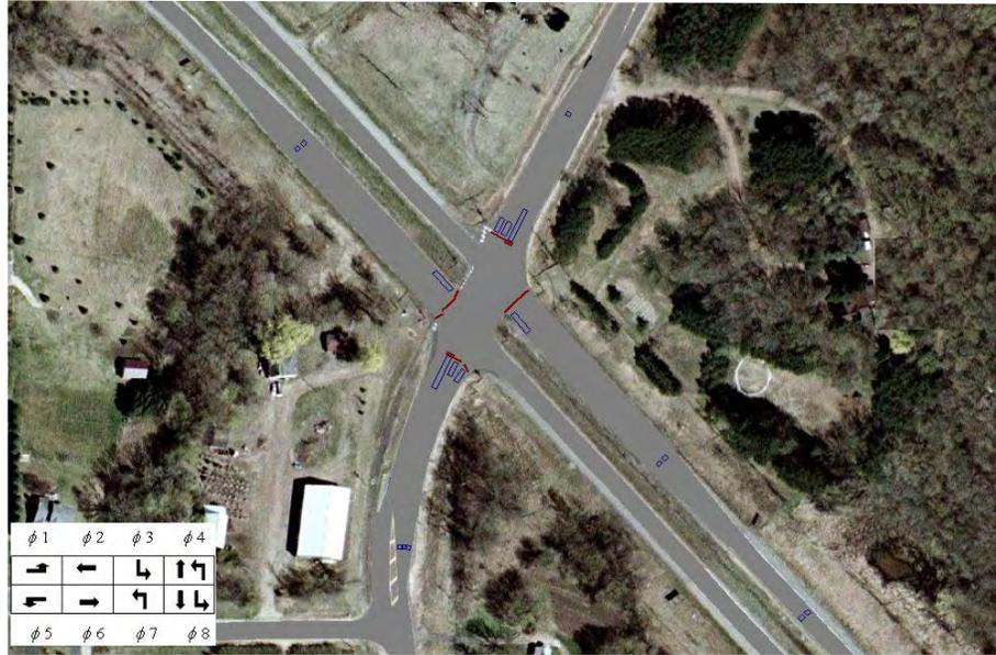
Traffic data gathered using detectors at this high-speed, signalized isolated intersection was used in simulations of different signal control systems in the lab.
