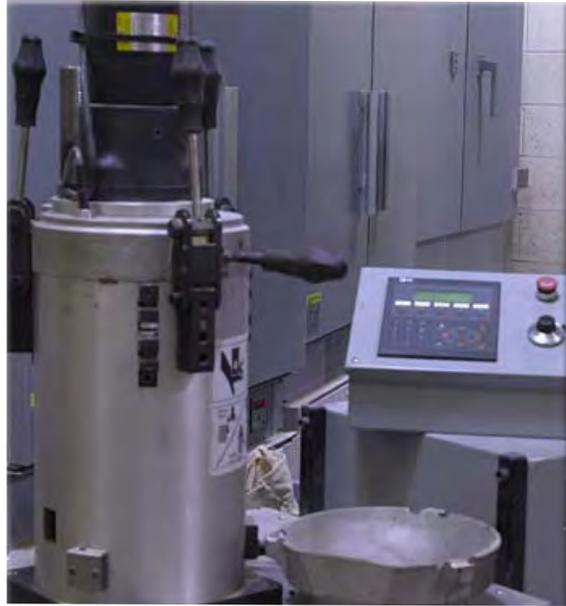
To evaluate hydraulic, mechanical and leaching characteristics, researchers used a gyratory compactor to prepare specimens at maximum density, which more realistically approximates real-world pavements than specimens prepared using more common methods.
