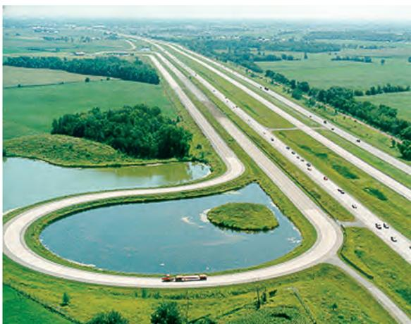
**SP&R funding provides increased opportunities to use the MnROAD cold-region testing laboratory, a unique platform for testing road-building materials and designs. MnROAD features two road segments—3.5 miles of mainline highway and 2.5 miles of low-volume roadway—divided into 52 test cells.**
