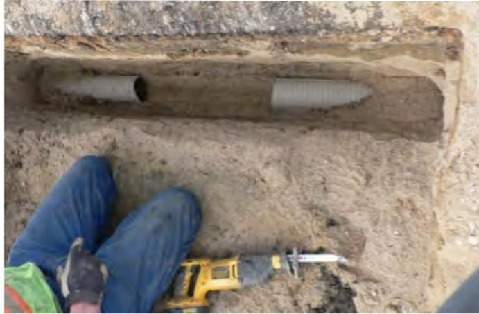
Researchers cut out sections of edge drain pipes to evaluate sediment composition.
