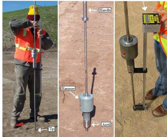
A DCP estimates soil strength by measuring how far a driven metal cone penetrates the ground.
