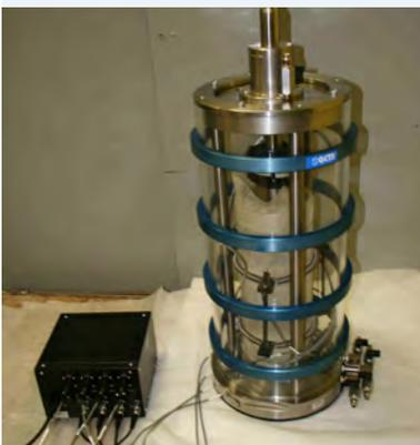
A triaxial pressure chamber was used to determine the resilient modulus of specimens by measuring their compaction under various loads.
