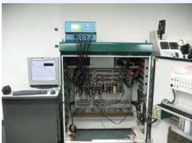
Investigators conducted lab simulations using a personal computer, controller cabinet and signal controller.
