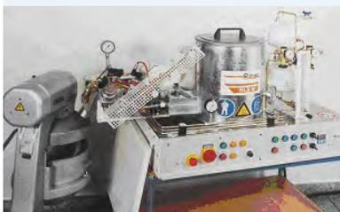
Introducing moisture into a stream of hot asphalt creates a foam that mixes well with aggregates.
