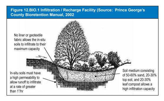
facility type is suitable for areas and land uses that are expected to generate nutrient runoff (i.e.; residential and business campuses) that can be infiltrated and captured by the facility. Fresh mulch rather then aged shredded bark mulch can be used to enhance denitrification processes.
