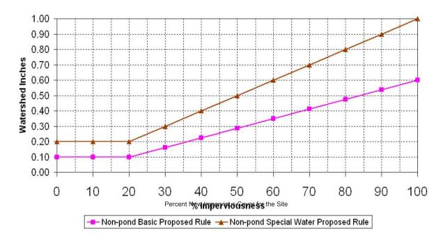
The four water quality sizing rules are compared against each other in Figure 10.6. An even higher degree of phosphorus removal may be needed to protect the most sensitive lakes and susceptible wetlands. Recommended guidance on sizing BMPs for these special receiving waters is provided in Sections IX Lakes and XII Wetlands, respectively.
