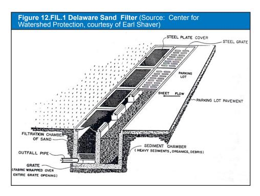
volume is temporarily stored in both the first and second chambers. Flows in excess of the filter's capacity are diverted through an overflow weir. Filtered runoff is collected, using perforated underdrains that extend into the third "overflow" chamber. See Appendix D for design drawing.
