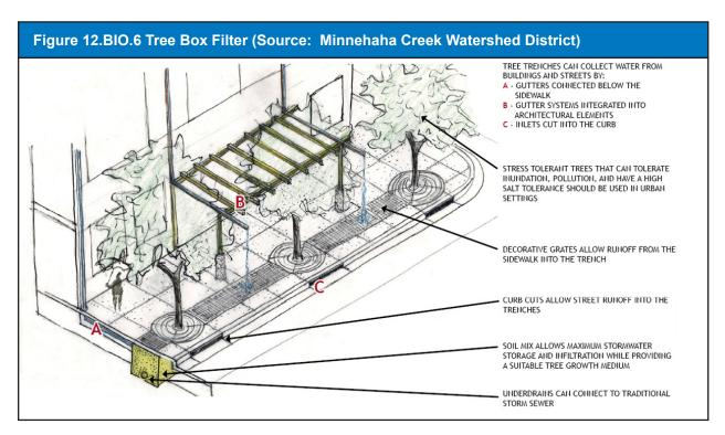
➤ Tree Pits / Tree Box Filters – tree Pits and tree box filters afford many opportunities for bioretention. Designs vary widely from simple "tree pits", used for local drainage interception to more formal tree box filters, which are a useful tool for highly urbanized streetscapes.
