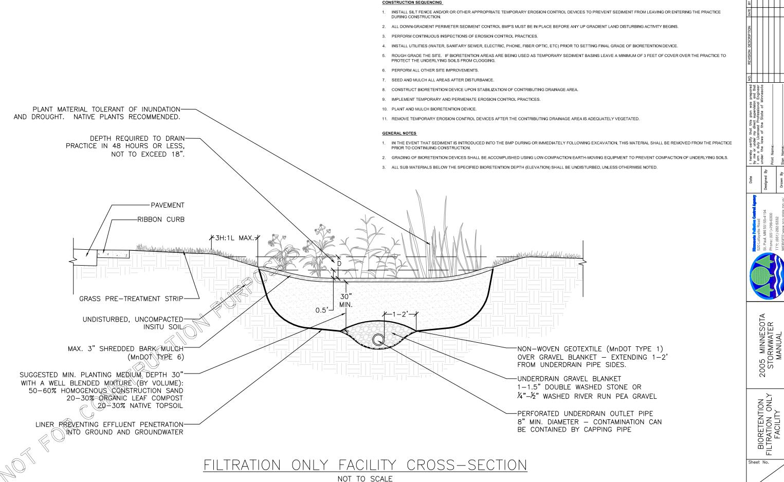
BIORETENTION FILTRATION ONLY FACILITY Sheet No. Appendix D-BIOCAD
