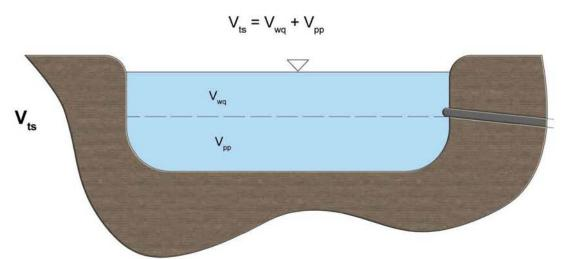
\*V<sub>wq</sub> equals 1/2" for normal receiving water and 1" for CGP special waters
