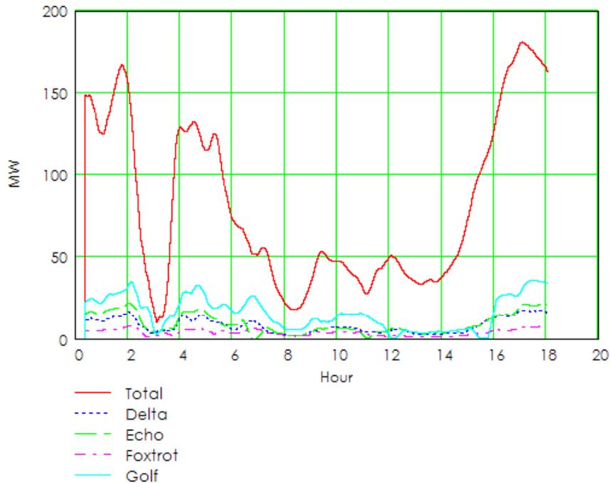
Figure 46: Trend characteristic extracted from raw data of Figure 44 with a 20 minute time averaging period.
