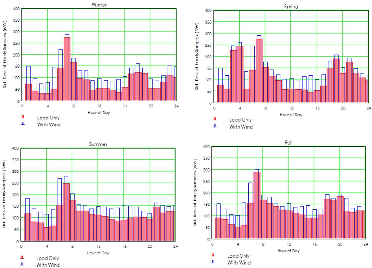
Figure 56: Standard deviation of ramping requirements with and without wind generation, by hour of day and season.
