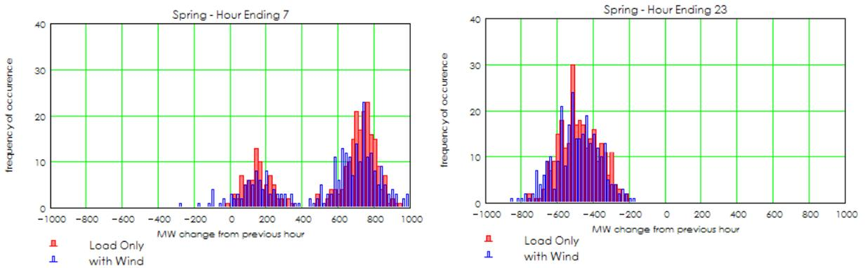
Figure 58: Ramping requirement with and without wind generation for selected hours during spring.
