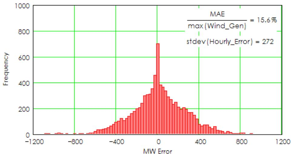
Figure 70: Forecast error statistics for 2003 wind generation time series.
