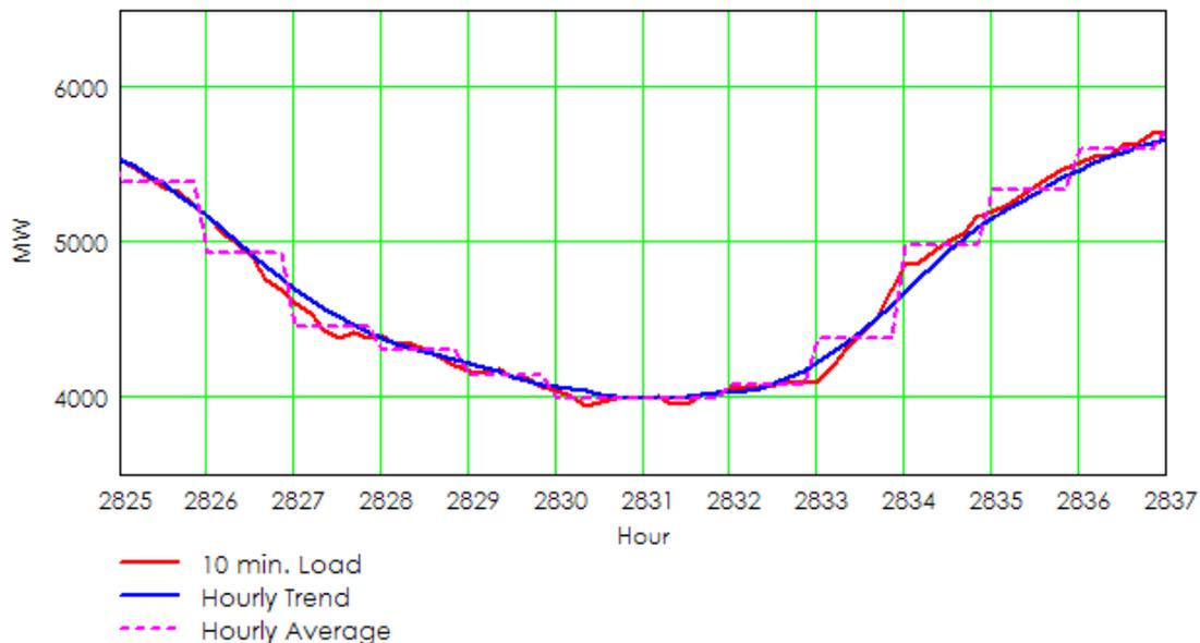
Figure 82: 12-hour load time series showing high-resolution data (red), hourly trend (blue), and hourly average value (magenta).
