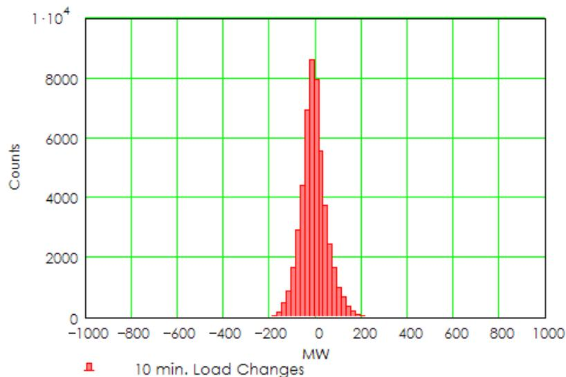
Figure 78: Distribution of 10 minute changes in system load.
